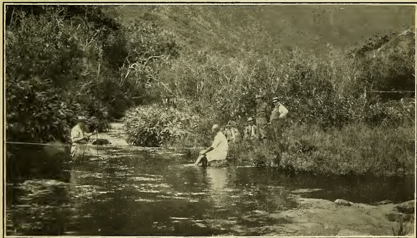
B. VELOCITY-AREA GAGING STATION, WAIHOLE STREAM, OAHU.
