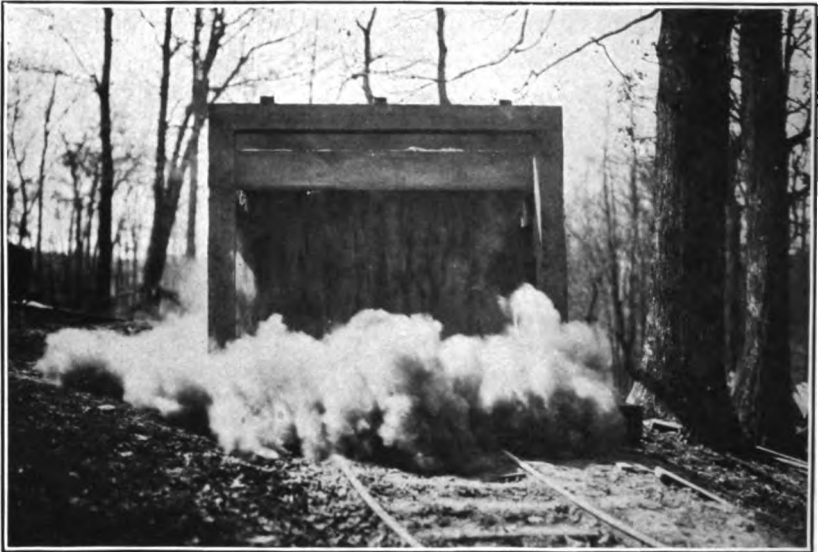
1. CLOUD OF DUST CAUSED BY THE DISCHARGE OF ONE OF THE TROUGHS OF A TROUGH BARRIER IN A MINE ENTRY.
