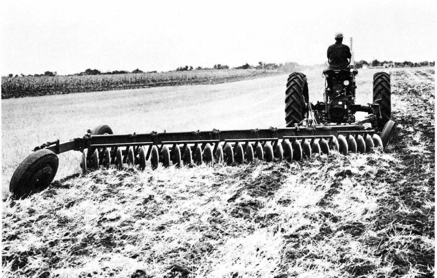
Figure 8—Trailing-type, multiple gang, vertical disk plow. (Courtesy of International Harvester Co.)
