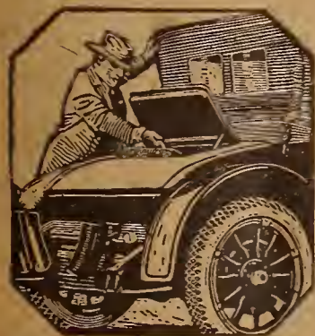
At Left: By lifting the small cover in the rear deck, space is given for carrying small articles such as doctor's cases, sample cases, etc.
