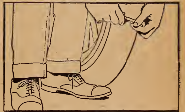
LET THE TIRE STAND 12 HOURS—OR LONGER. When thoroughly dry and hard, trim off the ragged edges of the repair with a wet knife. The job is complete, the tire is saved, and the repair will last fully as long as the rest of the tread.
