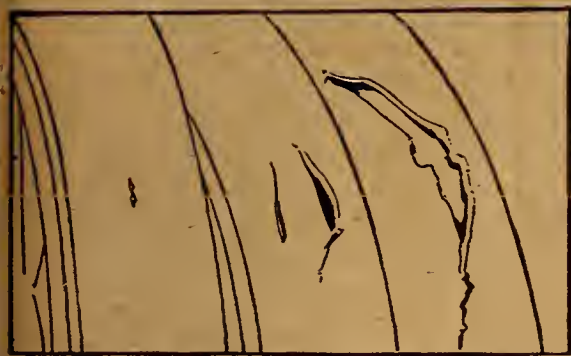
HOW TREAD CUTS GROW. If your tire receives a small tread cut that is not attended to, this cut will soon grow in size, causing quick ruin to the tire as shown above. It is wise to have your Goodyear Service Station Dealer repair these cuts immediately, or show you how to do it yourself with the Goodyear Tire Putty Outfit.
