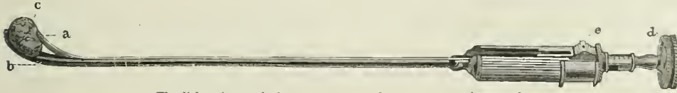
The lithotrite: a b , jaws; c , stone; d , screw; e , spring catch.
