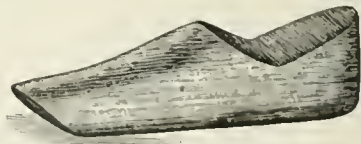
FIG. 5.—Showing the block of wood over which a rubber foot is molded.
