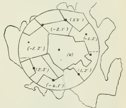
FIG. 2.—Minot's Ledge, as prepared to receive the foundation-stones.
