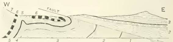
FIG. 2.—Section of folded and faulted beds of the Appalachian systems in Eastern Tennessee (after Campbell). Arrows show the directions of motion along the fault plane. Formation 2, originally underlying 3, and overlying 1, is by the dislocation made to rest on the broken ends of 1, 2, 3, and 4.
