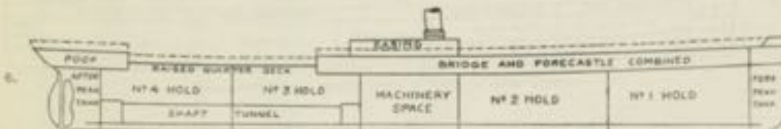
VESSEL WITH A POOP, A RAISED QUARTER DECK, AND A BRIDGE AND FORECASTLE COMBINED. PART AWNING DECK.
