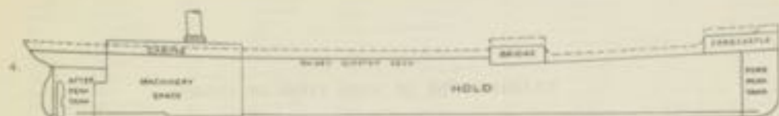
VESSEL WITH A RAISED QUARTER DECK, A SHORT BRIDGE, AND A FORECASTLE. WELL DECK.
