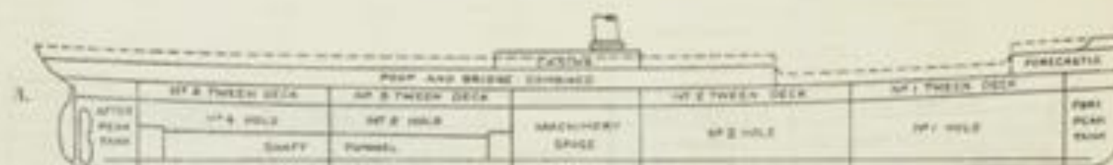
VESSEL WITH A COMBINED POOP AND BRIDGE AND A FORECASTLE. WELL DECK
