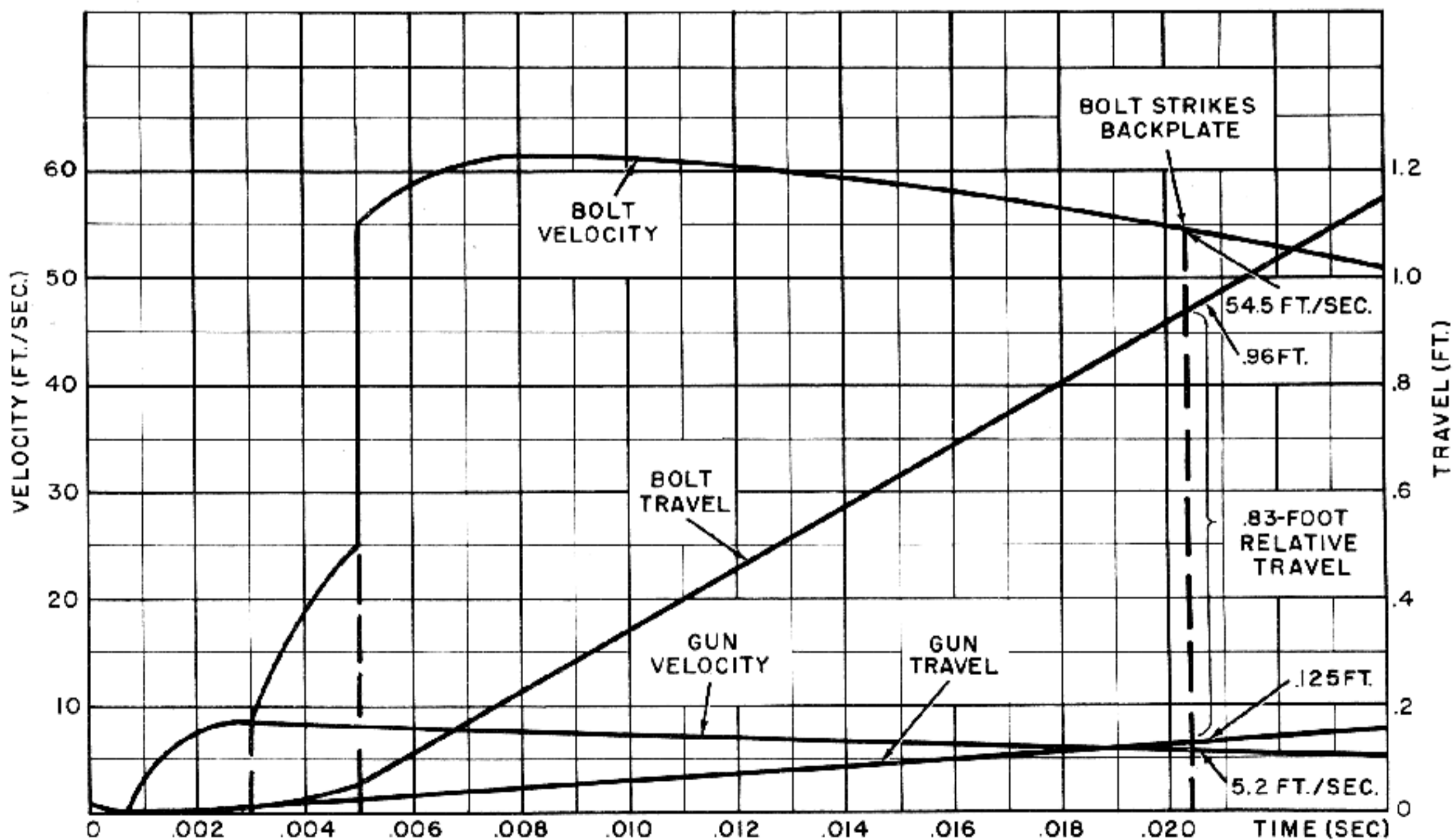
Figure 3-33. Time-Travel and Time-Velocity Curves for Gun and Bolt Up to Instant Bolt Strikes Backplate.
