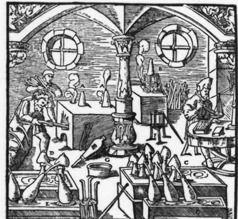
A—AMPULLAE ARRANGED IN THE VESSELS. B—AN AMPULLA STANDING UPRIGHT BETWEEN IRON RODS. C—AMPULLAE PLACED IN THE SAND WHICH IS CONTAINED IN A BOX, THE SPOUTS OF WHICH EACH FROM THE OPERCULA INTO AMPULLAE PLACED UNDER THEM. D—AMPULLAE LIKEWISE PLACED IN SAND WHICH IS CONTAINED IN A BOX, OF WHICH THE SPOUT FROM THE OPERCULA EXTENDS CROSSWISE INTO AMPULLAE PLACED UNDER THEM. E—OTHER AMPULLAE RECEIVING THE DISTILLED OILS AND LIKEWISE ARRANGED IN SAND CONTAINED IN THE LOWER BOXES. F—IRON TRIPOD, IN WHICH THE AMPULLA IS USUALLY PLACED WHEN THERE ARE NOT MANY PARTICLES OF GOLD TO BE PARTED FROM THE SILVER. G—VESSEL.
