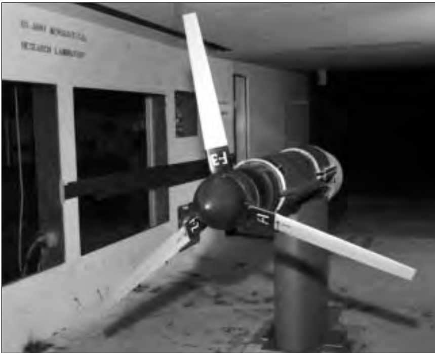
Figure 28. Performance tests of 5-ft. diameter proprotor in the Army 7- by 10-ft. wind tunnel at the Ames Research Center. (Ames Photograph AC98-0209-4)
