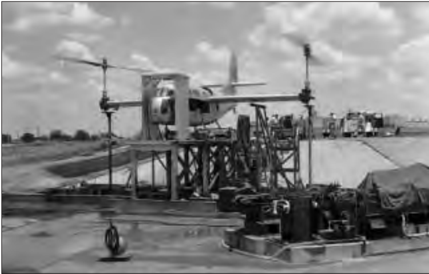
Figure 20. Tiedown tests of the XV-3 with protective shields at Bell in July, 1957. (Bell Photograph 220955)
