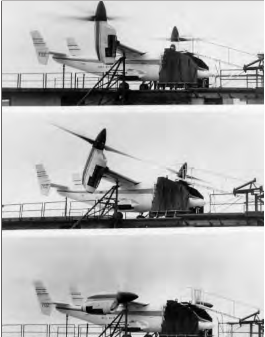
Figure 44. Initial Bell tiedown showing metal protective shields. (Bell Photograph 240178)
