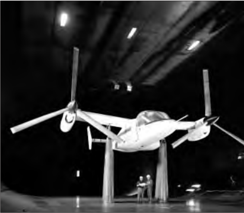
Figure 45. XV-15 in the Ames Research Center 40- by 80-ft. wind tunnel. (Ames Photograph A78-0579-3)
