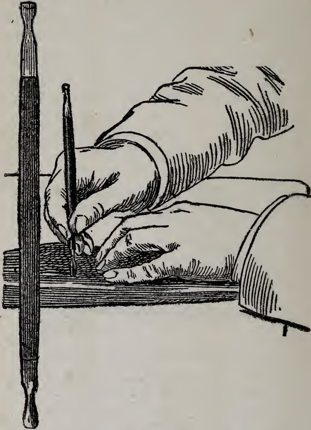
FIG. 27.—SECOND POSITION OF OUTLINING TOOL
