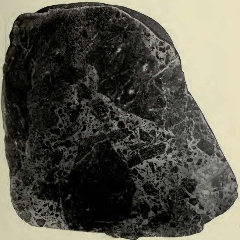
FIG. 1. Chert breccia cemented by zinc blende.
