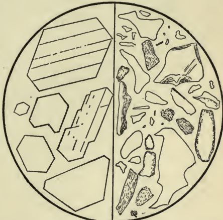
FIG. 29.—Showing, on the left, the mineral kaolinite as seen under the microscope, and on the right, washed kaolin.
