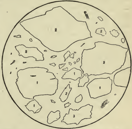
FIG. 26.—Showing angular outlines of residuary particles from decomposed gneiss. 1, mica; 2, feldspar; 3, quartz.
