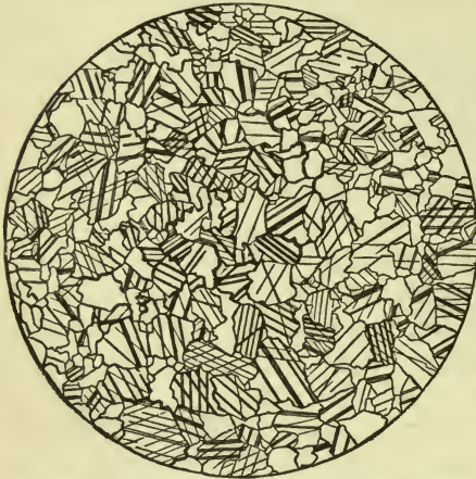
FIG. 14.—Microstructure of crystalline limestone (marble).
