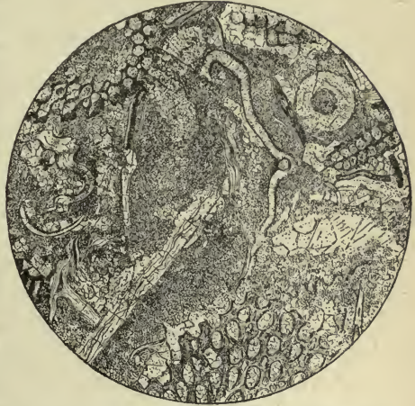
FIG. 12.—Microstructure of fossiliferous limestone.
