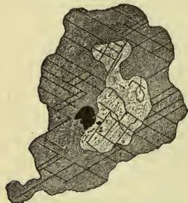
FIG. 1.—Augite partially altered into hornblende.
