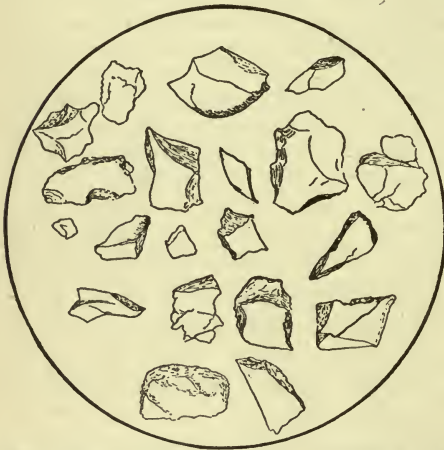
FIG. 28.—Showing angular character of quartz particles in decomposed gneiss.
