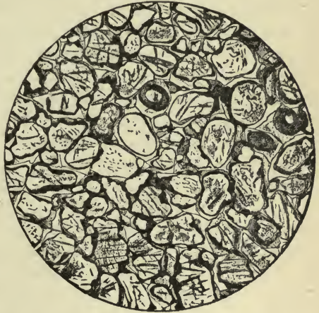
FIG. 13.—Microstructure of quartzite, showing secondary deposit of silica about the original quartz grains.
