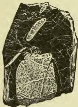
FIG. 8.—Pyroxene partially altered to serpentine.
