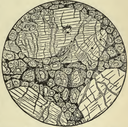
FIG. 5.—Microstructure of porphyritic lherzolute, partly altered into serpentine.
