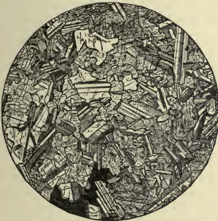
FIG. 4.—Microstructure of diabase.
