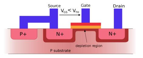
The 'metal' in the name MOSFET is now often a misnomer because the previously metal gate material is now often a layer of polysilicon (polycrystalline silicon). Aluminium had been the gate material until the mid 1970s, when polysilicon became dominant, due to its capability to form self-aligned gates. Metallic gates are regaining popularity, since it is difficult to increase the speed of operation of transistors without metal gates.
