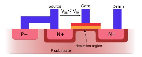
when the gate voltage VGS is below the threshold for making a conductive channel; there is little or no conduction between the terminals source and drain; the switch is off. When the gate is more positive, it attracts electrons, inducing an n-type conductive channel in the substrate below the oxide, which allows electrons to flow between the n-doped terminals; the switch is on.
