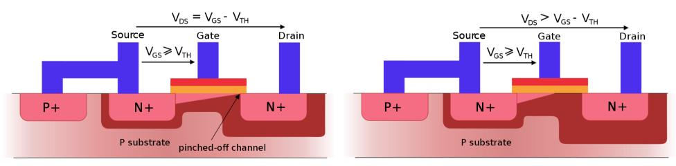
Saturation mode at point of pinch-off
