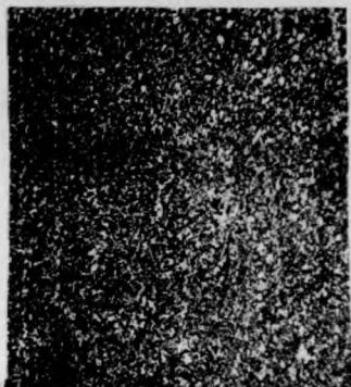
FIG. 171.—High-speed Steel, Annealed. \times 200 . (MacFarland.)
