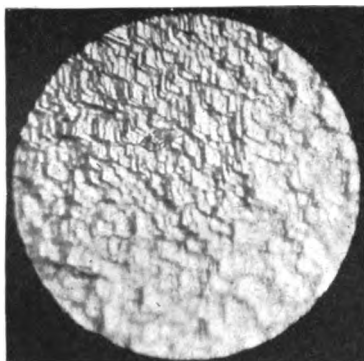
FIG. 2.—Artificial markings on face of a diamond, produced by partial combustion.
