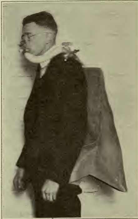
Fig. 180.—The Douglas bag method for determining the respiratory exchange. The arrangement of mouthpiece, valves, and connecting tubes shown here has been found to be more convenient than that recommended by Douglas.
