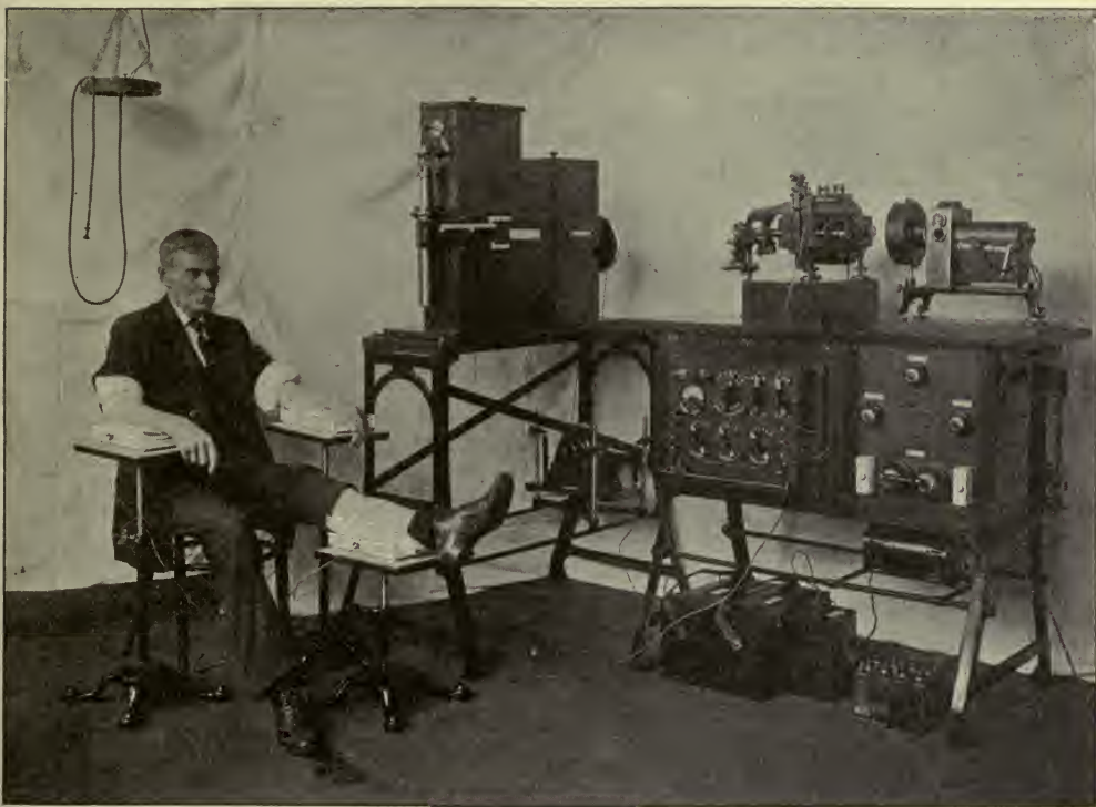
Fig. 81.—Electrocardiographic apparatus as made by the Cambridge Scientific Materials Co. Contact electrodes are shown, but the immersion electrodes described in the context are preferable.
