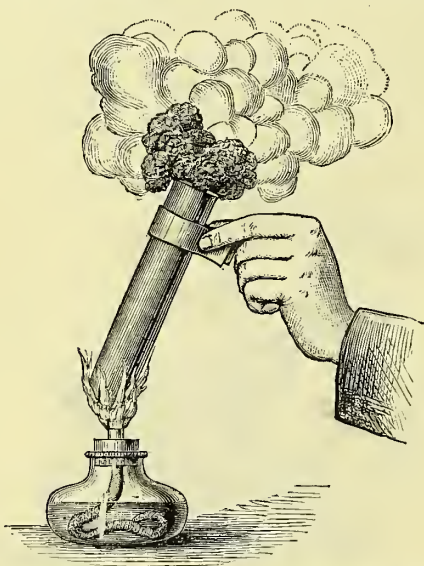
Fig. 2.—Experiment showing the Conversion of Sugar to Charcoal.
