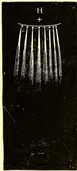
Fig. 7.—Artificial Aurora produced in an Exhausted Vacuum Tube by the Discharge of 14,400 Cells of the large Battery.
