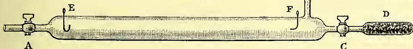
Fig. 3.—A Vacuum Tube of the Form employed by Dr. De la Rue in his Experiments with Cocks capable of being opened and closed at A, B, and C, with an Absorption Chamber at D, and with pieces of Platinum or Aluminium Wire inserted through the Glass, and hermetically cemented to it at E and F, so that their Points are 29 inches asunder.
