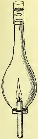
Fig. 8.—A Glass Tube furnished with Flame Sieves, in which a common Candle may be burnt.
