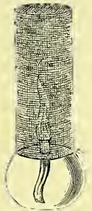
Fig. 9.—A Cylinder of Gauze surrounding a Lamp Flame.
