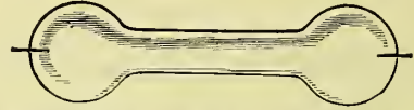
Fig. 5.—A Vacuum Tube constructed so that there is a Comparatively Narrow Central Part intervening between wide bulb-shaped ends.
