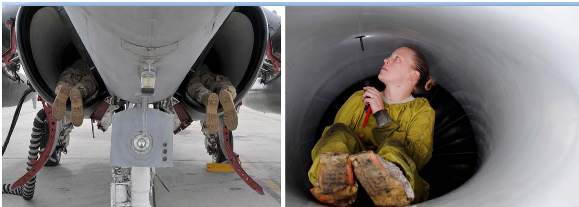
Figure 8. Inlet Inspection of E/A 6B and F-16. From [17]
