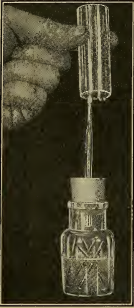
FIG. 17. — Making hydrogen. The bottle contains five nails and weak sulphuric acid. To the right of the flame of hydrogen at the tip of the glass tube are two drops of water formed by the union of the hydrogen coming out of the bottle and the oxygen in the air.
