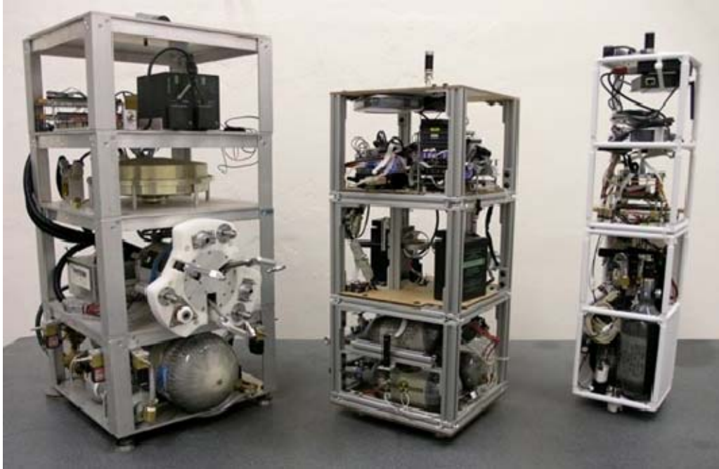
Figure 1. Three Generations of Spacecraft Simulators at the NPS Spacecraft Robotics Laboratory (first, second and third generations, from left to right)
