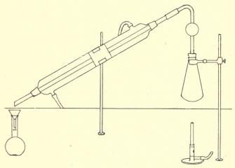
tions of water should be added drop by drop, and the flask shaken between each addition, in order to avoid foaming. When the soap is dissolved, 5 c. c. of the dilute sulfuric acid are added, a piece of pumice dropped in and the liquid distilled until 110 c. c. have been collected. The condensing tube should be of glass,
