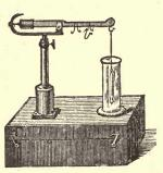
Westphal balance. This is a delicate steelyard with a counterpoised plummet, displacing 5 c. c. The plummet being immersed in the milk the equilibrium is restored by weights, the value of which can be directly expressed in figures for the specific gravity.
