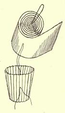
the milk to be tested, run on to the upper part from a pipette. The milk is rapidly absorbed by the paper and none filters through the cap. It is then dried in a water oven for an hour or two.
