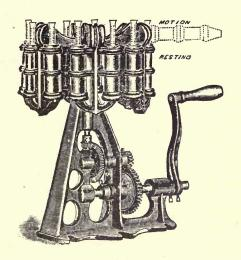
The test-bottles, the form of which is shown in the cut, have a capacity of about 30 c. c., and are provided with a graduated neck, each division of which represents one-tenth per cent by weight of butter-fat.
