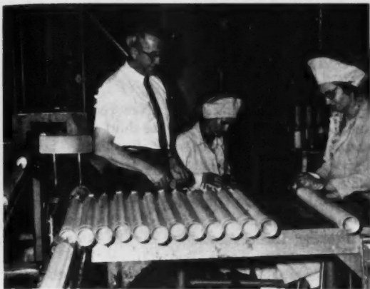
TOP MARCH CHAMPION —Jack Doyle, an ordnanceman at the U.S. Naval Ammunition Depot, McAlester, Okla., watches as workers install his brainchild—a shunting wire to prevent ignition, during shipment, of the "Mighty Mouse" air-to-ground rocket. Doyle's wire cost a nickel, compared to the forty-cent item it replaced. Savings: $2,098,560 on first-year procurement. Award (initial): $1,000. ( Navy photo )
