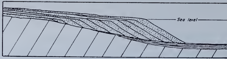
FIG. 3. The delta terrace redrawn from Dunbar and Rodgers (1957, p. 47). Topset, foreset, and bottomset beds are shown to develop when a sediment-laden river enters a quiet body of water. Such delta terraces are common geomorphic forms; they should not be confused with the entirely hypothetical wave-built terrace. Note especially that the nick-point is at water level and not below; wave action would tend to modify or destroy the delta terrace. A rising water level would drown it, producing a feature which might erroneously be interpreted as a wave-built terrace.
