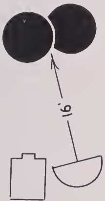
Figure 43. The S:L ratio was 100:800. Fill-in with one Wabash "25" at 16 feet. Bulb should have been slightly closer, as contrast remains a little too great.
