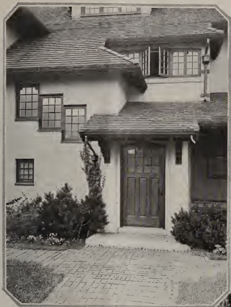
The breaking of the roof lines and a staggered stair window arrangement will effectually give interest and variety to an entrance
