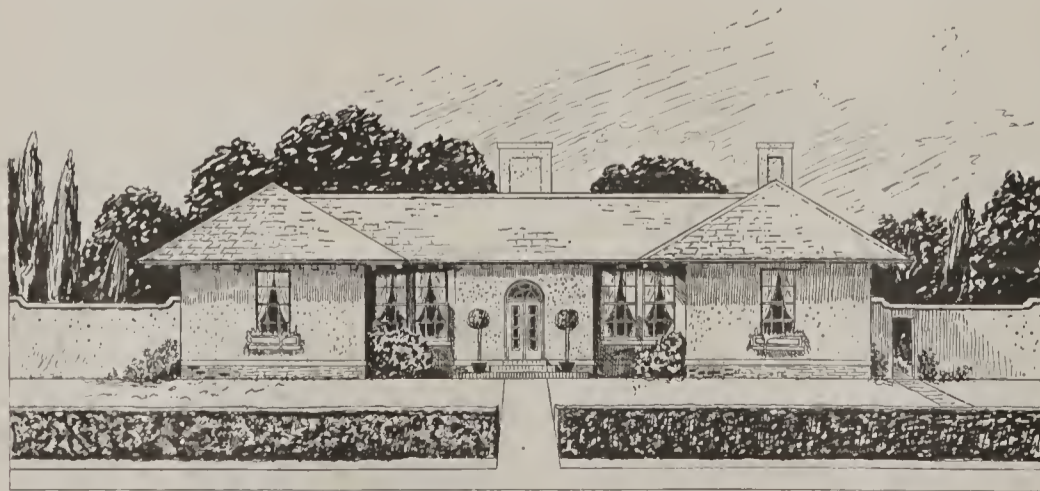
The outside walls are stucco over hollow tile, metal lath or mastic board. Chimneys of rough brick stuccoed. The roof is covered with heavy split cypress shingles stained green or brown
