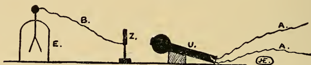
Fig. 34.—Experiment showing ultra-violet rays discharging a piece of zinc. U , ultra-violet lamp; Z , zinc; B , wire connecting zinc with electrode E . 2
