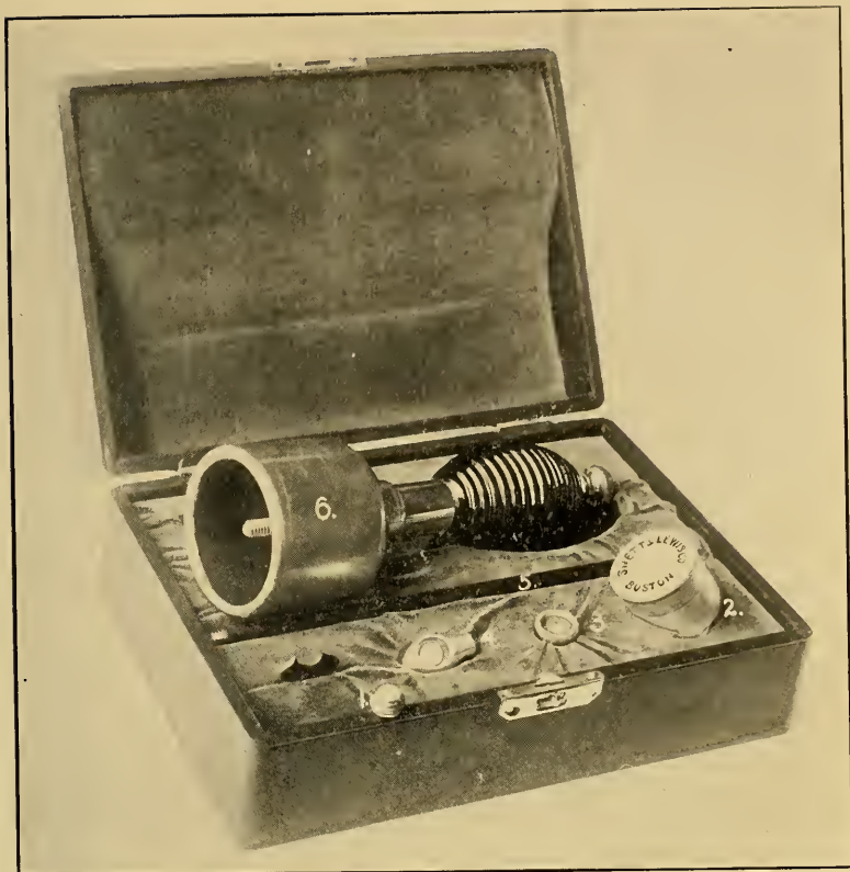
Fig. 52.—1, brass containing receptacle for radium; 2, box for containing this receptacle when carried in pocket; 3 and 4, applicators of solid silver; 5, handle for the same; 6, applicator made of lead to which No. 3 can be attached.
