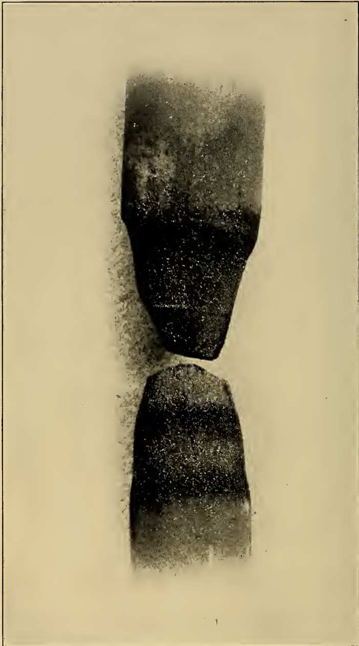
Fig. 1.—Carbons used in clinical work with a 25-ampère arc. The upper or positive carbon shows the crater-like depression, the lower or negative carbon the nipple-like projection. The area of incandescence is clearly shown as well as the disintegrating action upon the carbons under the double influence of volatilization and oxidation.
