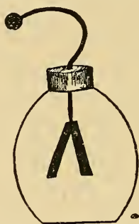
Fig. 33.—Electroscope with polished zinc ball, for showing the effect of ultra-violet rays. 1
