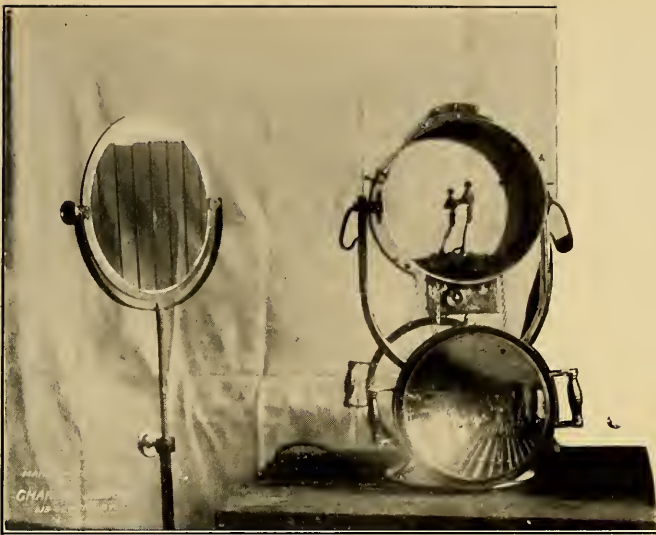
Fig. 21.—Marine Searchlight, with Blue Glass Screen.
