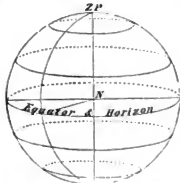
FIG. 32.—Showing that the true horizon of a pole is the equator.
