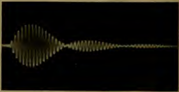
FIG. 2.—Beats in the Oscillatory Discharge of the Secondary of a Coupled Circuit. From a photograph by Prof. J. Zenneck. From "A Treatise on Electricity."
