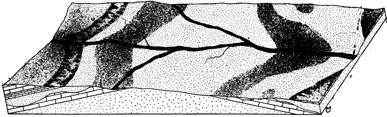
Fig. 31. Block diagram showing the courses of the streams in a final stage of stream adjustment in a first cycle of erosion.
