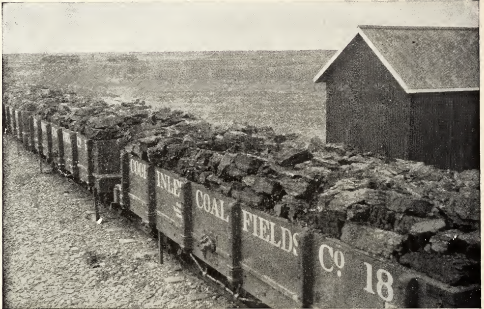
ALASKA LIGNITE COAL, EXPOSED FOR THREE YEARS TO WEATHERING AND SHOWING RESISTANCE
