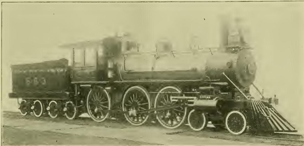
TEN-WHEELED LOCOMOTIVE, BUILT BY THE BROOKS LOCOMOTIVE WORKS FOR HIGH-SPEED SERVICE ON THE LAKE SHORE & MICHIGAN SOUTHERN RAILWAY.
