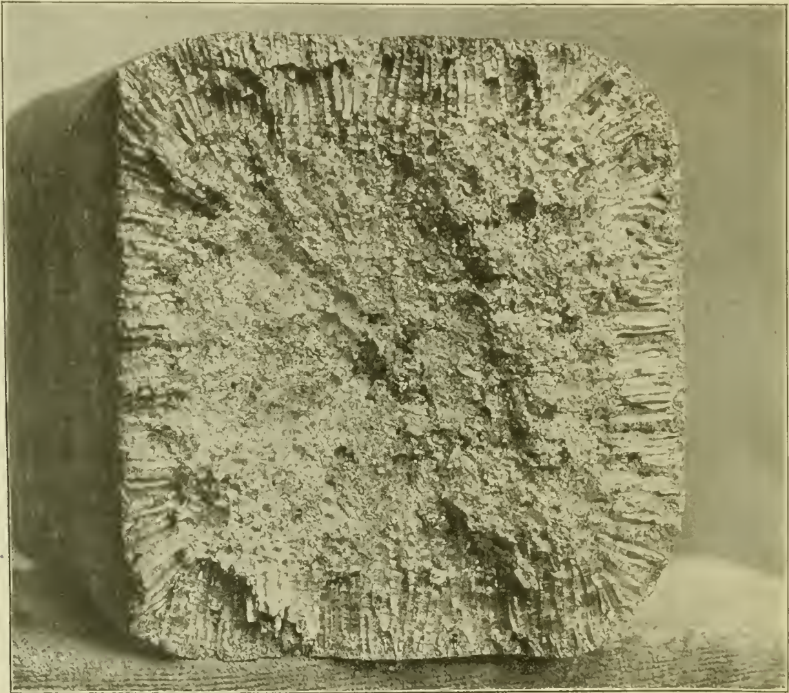
FRACTURE OF OPEN-HEARTH STEEL INGOT. AREA, 6\frac{1}{2} IN. \times 6\frac{1}{2} IN.
