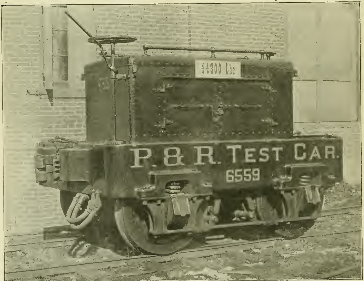
SCALE-TESTING CAR FOR PHILADELPHIA & READING RAILROAD.
