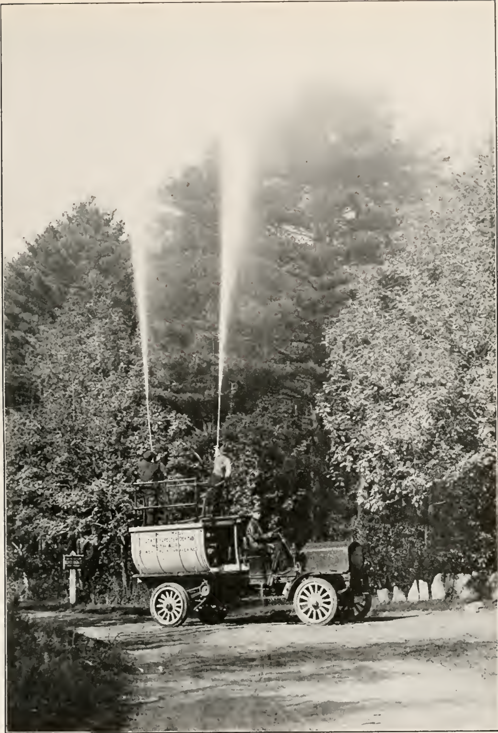
THE FIRST POWER-TRUCK SPRAYER EVER INVENTED. BUILT BY THE MASSACHUSETTS STATE FORESTER IN 1911 FOR SPRAYING IN THE GYPSY AND BROWN-TAIL MOTH WORK. THE WHOLE OUTFIT WAS DESIGNED AND BUILT FOR THIS WORK, AND PROMISES TO REVOLUTIONIZE THE QUESTION OF SPRAYING, PARTICULARLY ROADSIDE, PARK AND SHADE TREE WORK, IN COMBATING INSECT AND FUNGOUS DEPREDATIONS. IT CAN BE USED FOR FOREST FIRE WORK AS WELL. THE SAME ENGINE THAT PROPELS THE TRUCK ALSO IMPARTS THE POWER FOR SPRAYING.
