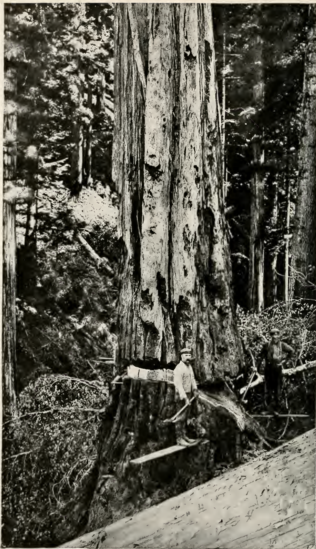
REDWOOD LOGGING. FELLERS MAKING THE UNDERCUT. AFTER THIS HAS BEEN DONE AND THE BARK CUT AWAY A SAW IS USED.
