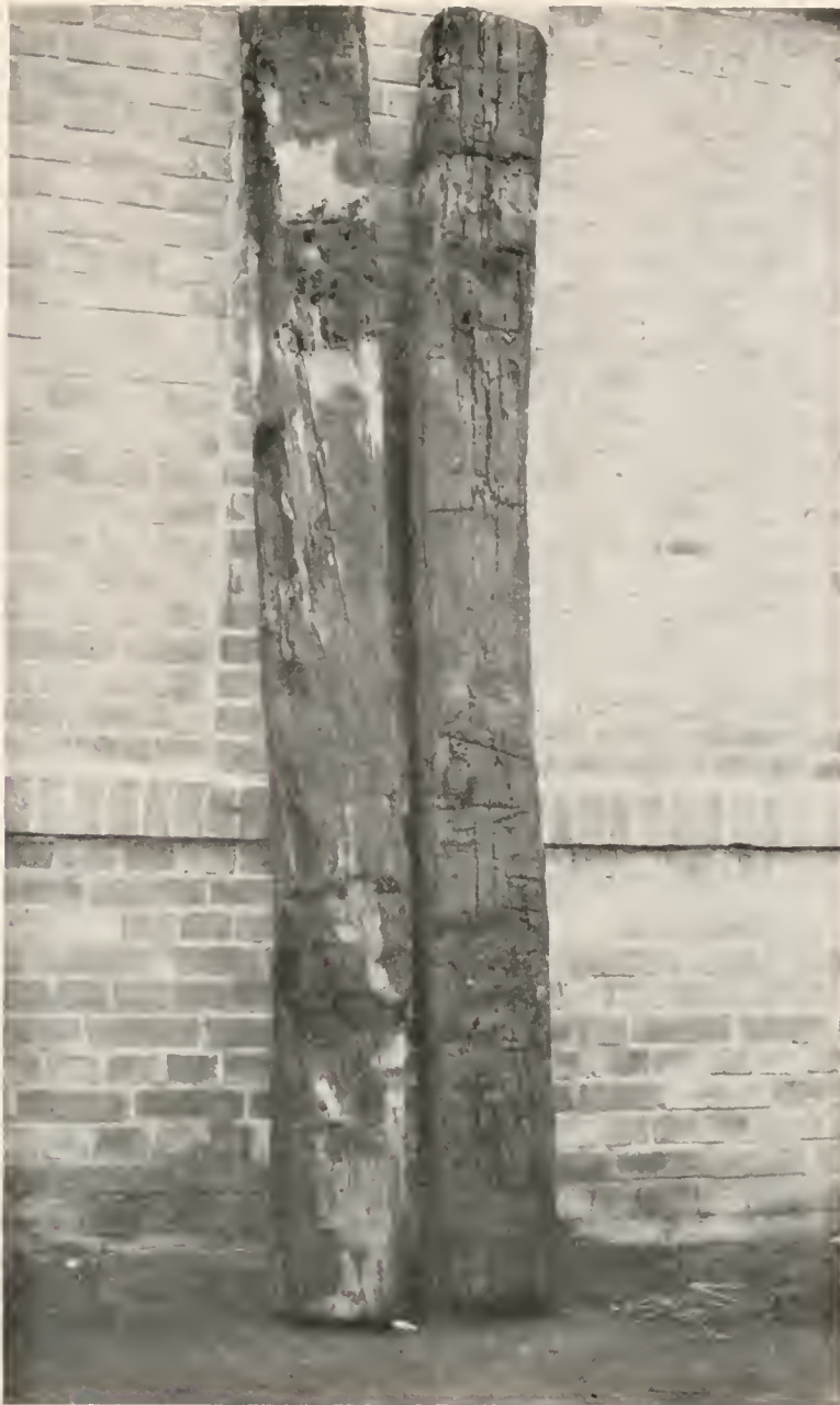
PINE TIES TAKEN FROM TRACKS OF PRUSSIAN STATE RAILWAY AFTER TWENTY-THREE YEARS' SERVICE. TREATED WITH ZINC CHLORIDE AND CREOSOTE.
