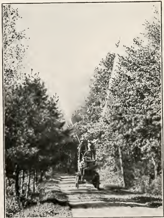
THE POWER-TRUCK SPRAYER IN ACTION, THROWING TWO STREAMS AND TRAVELING AT THE RATE OF 4 OR 5 MILES AN HOUR.
