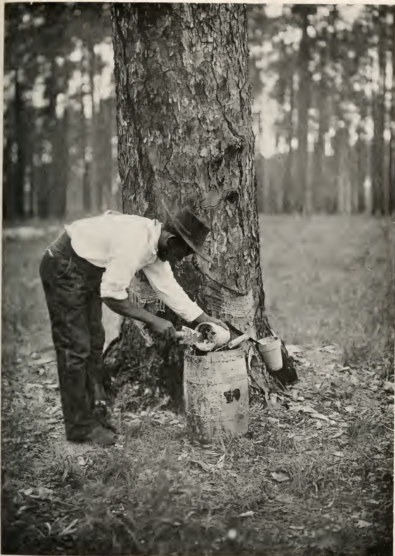
GATHERING CRUDE RESIN FROM WHICH TURPENTINE IS DISTILLED. CUP AND GUTTER SYSTEM, LONG LEAF PINE FOREST, FLORIDA
