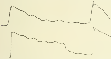
FIGURE 1.—About one half the original size. The lower tracing was taken from the trachea of the horse. The upper tracing was taken through the wall of the guttural pouch. The levers of the tambours rose and fell together, and the similarity of the tracings is marked.
