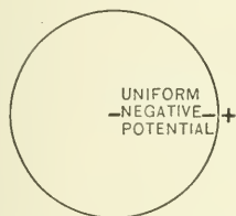
FIGURE 1. — Showing probable electrical condition of the cytoplasm during rest: a gradient of ca. 0.1 volt between outer and inner surfaces of plasma membrane; the potential within the cytoplasm practically uniform in all regions, and ca. 0.1 volt lower than the outer surface of the membrane. The cytoplasm is thus isoelectric — no gradient between its central and peripheral regions. 38
