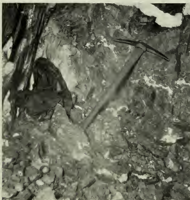
Face of drift, 170-ft. level, showing flat vein slightly faulted in mineralized zone, Matachewan mine.
