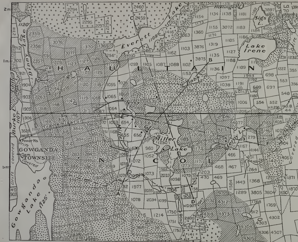
Geological plan of part of the Gowganda Silver Area, scale 3,000 feet to the inch, showing Sections in the vicinity of Miller Lake.
