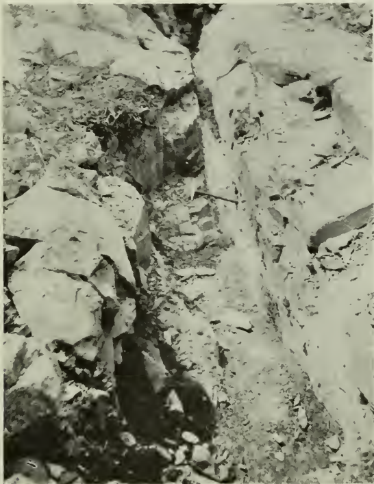
View on Symmes-Young claim, H.S. 351, containing massive smaltite and niccolite (7 inches in width at hammer). The rock is quartzite-conglomerate, Cobalt series.
