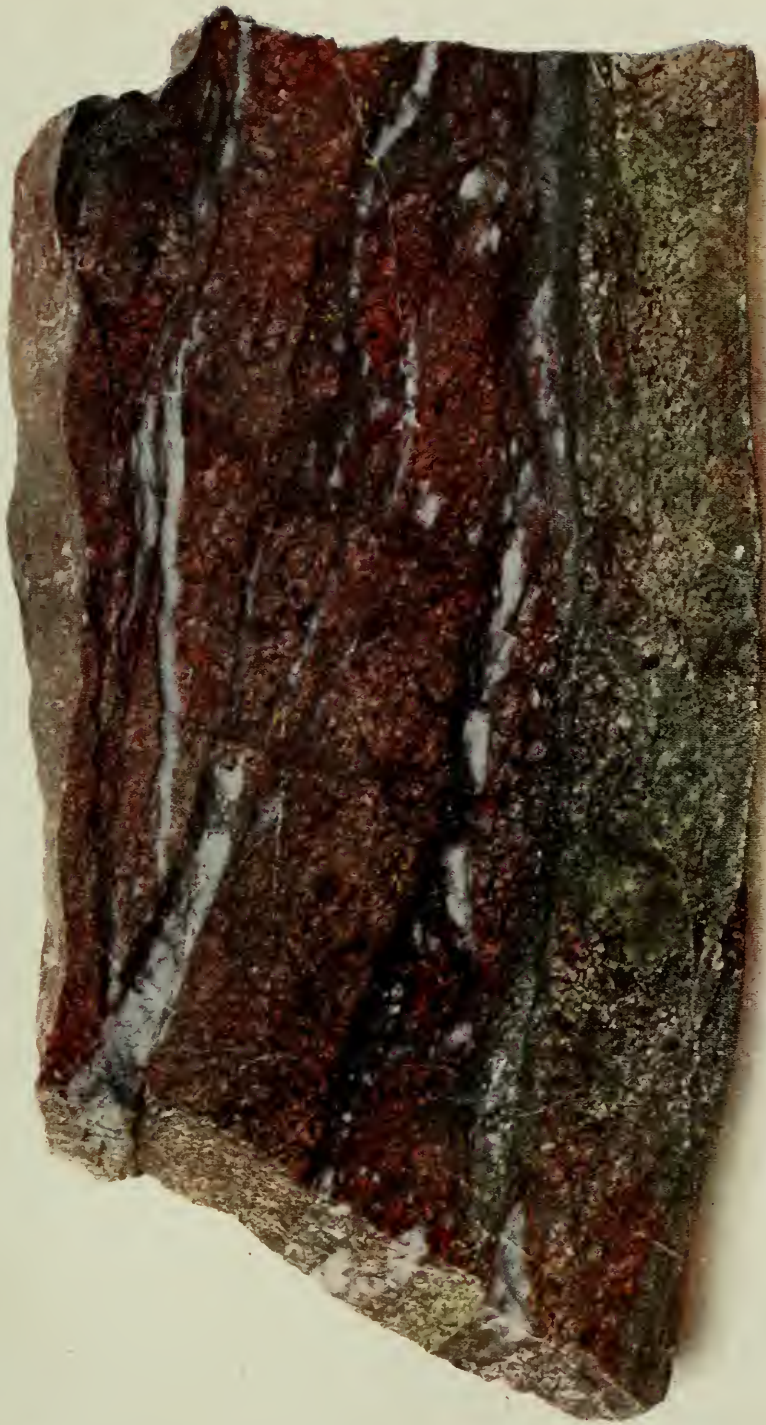
Polished Sample (Natural Size) of high-grade Gold Ore in Red Porphyry and Syenite, typical of the Kirkland Lake Area. From Kirkland Lake mine.
