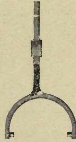
Outside of coupling rod
