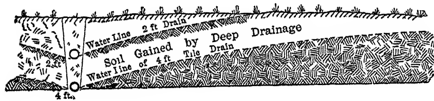
FIG. 19.—Effect of Depth of Drains on Open Soils.
