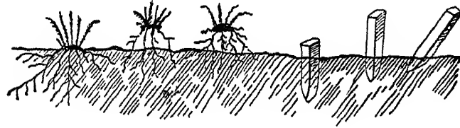
FIG. 2.—Heaving of Wet Soils.
