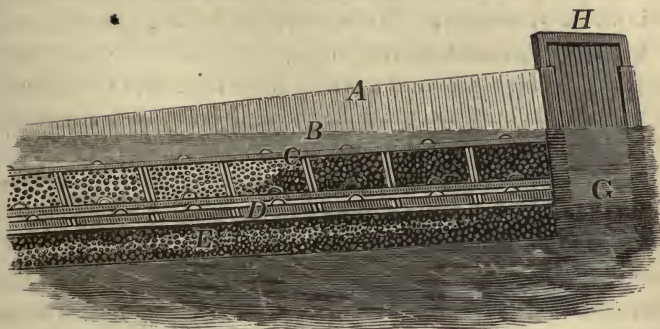
A. Top of Race. B. Water Level. C. Upper Screen, or Sieve. D. Under Screen. E. Bottom of Race. G. Supply Pond. H. Filtering Gate.
