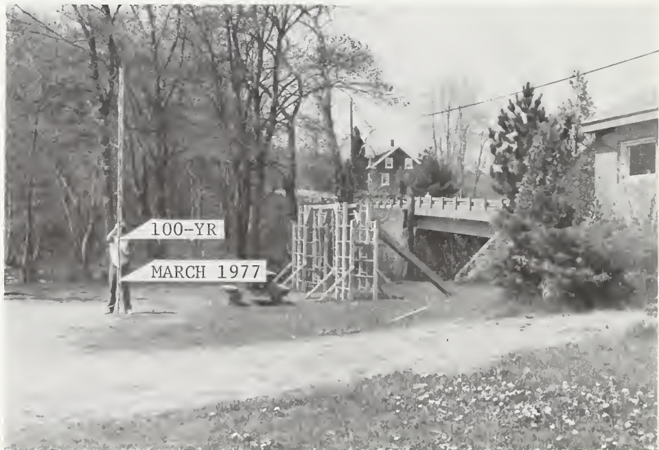
Ayer Park, on Seven Tree Pond - The estimated elevation of the 100-year flood is 45.4 feet NGVD or 4.9 feet above the ground at this point. The March 1977 flood shown has an estimated frequency of 25-years. (SCS photo)
