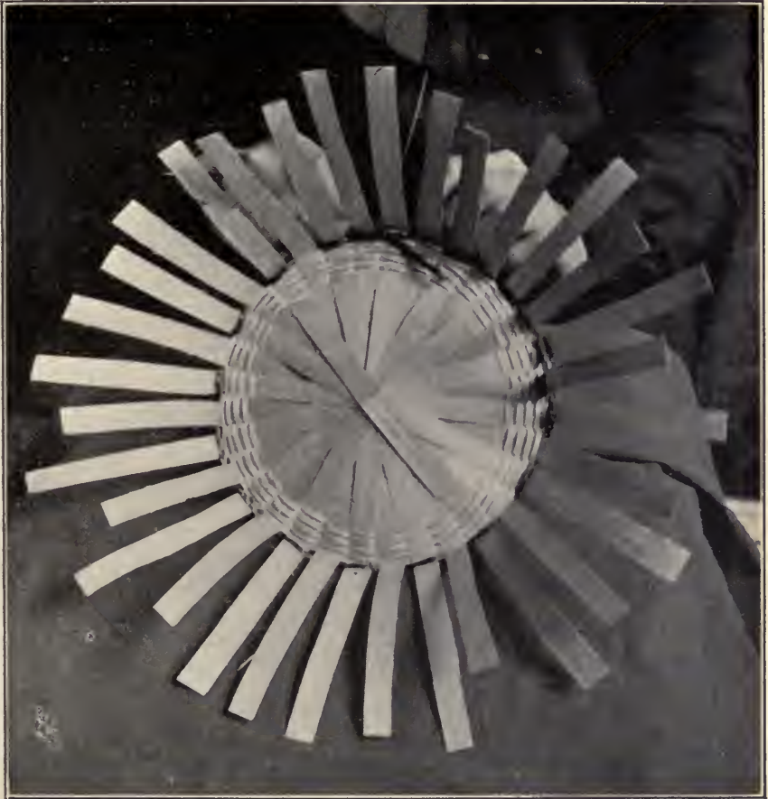
FIG. 143. SPOKES TURNED UP FOR SIDES.
