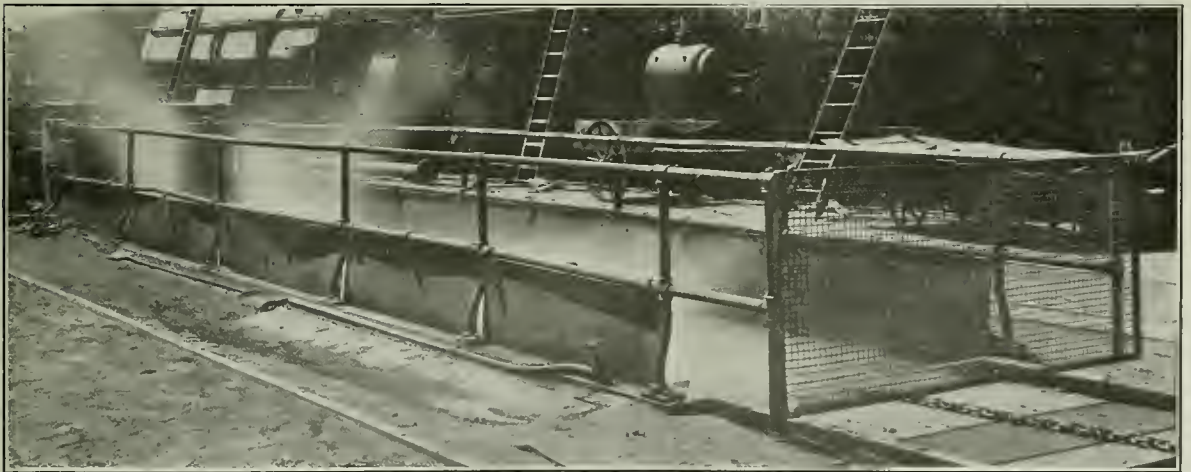
Fig. 9—Safety Railing Around the Lye Pit
