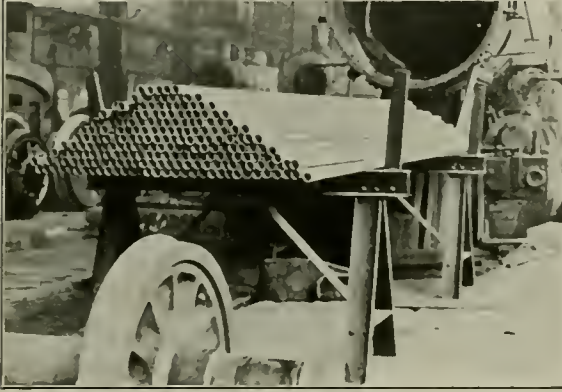
Fig. 1.—Tubes Removed from the Locomotive Are Piled on Special Standards
