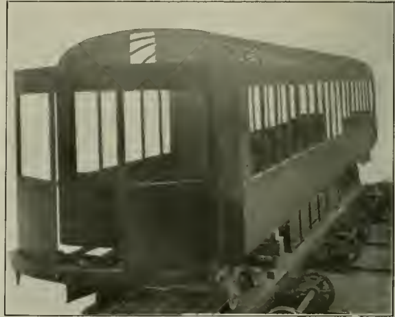
The Car Bodies and Their Appliances Are All Steel, Except for the Doors and Inside Finish
