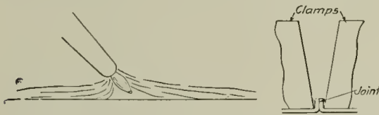
Arrangement of Clamps on Edison Joint which Use the Outer Flame as a Protection against Oxidation
