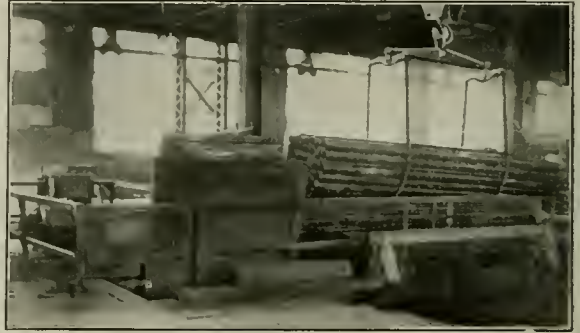
Fig. 3.—A Set of Flues About to Be Lowered Into the Pit Type Rattler
