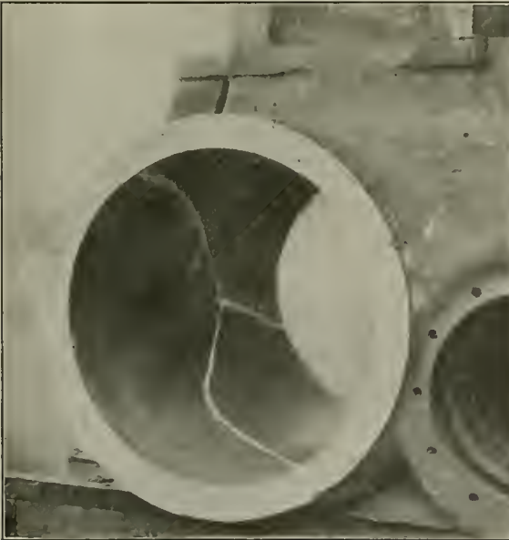
The Cylinder Casting After Welding and Boring
