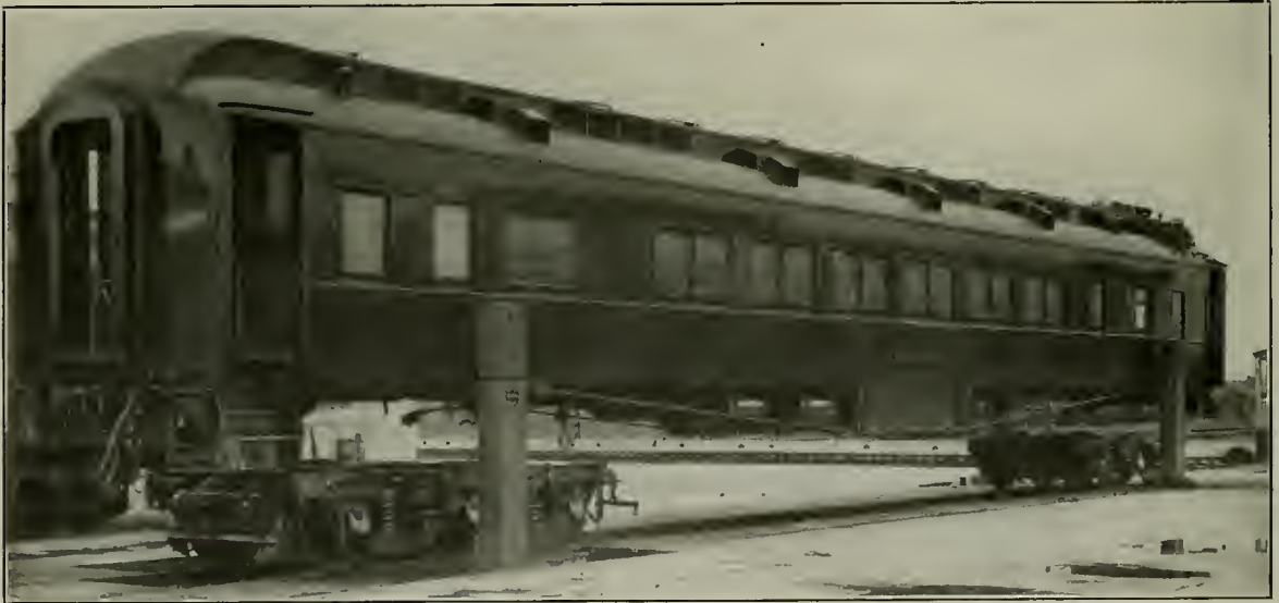
Coach Raised Sufficiently for the Trucks to Be Removed
