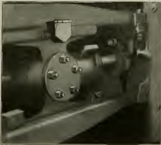
The Crosshead Pin Applied
