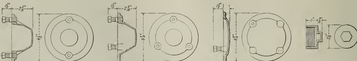
Caps for Protecting Triple Valves During Shipment
