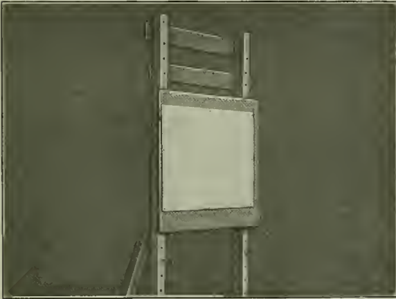
Screen for Recording the Movement of the Beams of Light Reflected by the Mirrors
