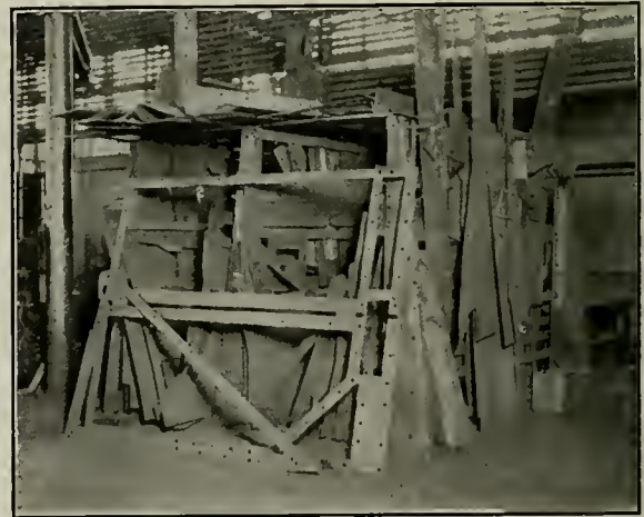
Sheet Metal Templets for Laying Out Parts of Steel Cars
