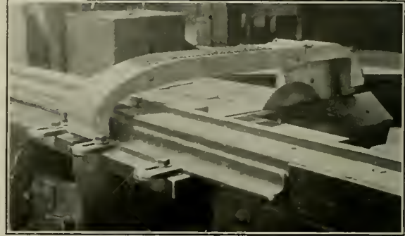
Fig. 5—Draw Cut Saw Guard in the Cabinet Shop
