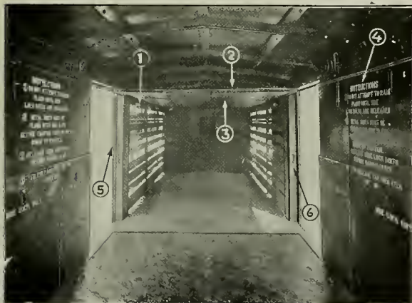
Fig. 2—One End of Car Arranged for Merchandise. (1) Safety Lock; (2) Movable Floor; (3) Showing Absence of Any Nails or Projections to Injure Live Stock; (4) Instructions for Operating Device; (5) Door water Seal; (6) Provision for Fastening Grain Doors.
