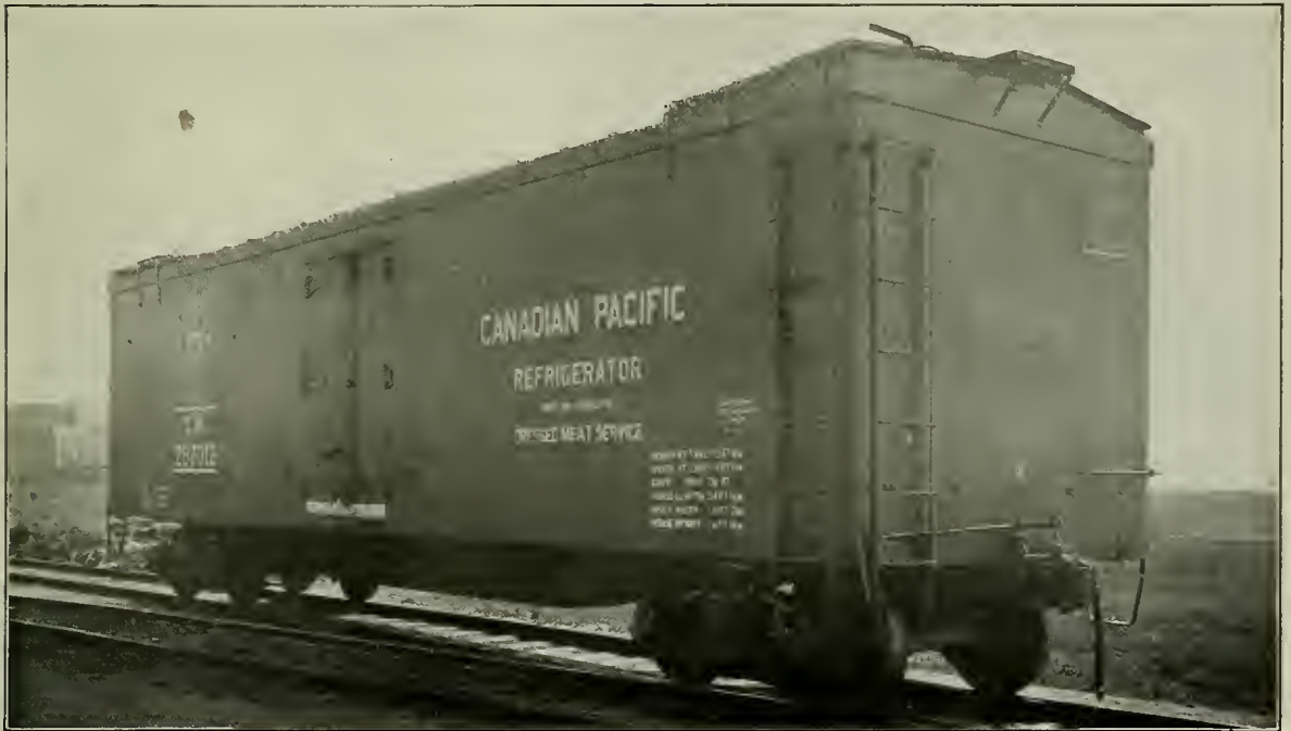
Steel Underframe Refrigerator Car with Brine Tanks and Ventilators, for the Canadian Pacific
