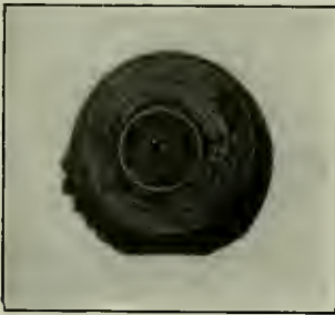
Water Glass Cock Opening Almost Closed by Scale
