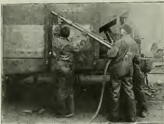
Pneumatic Rivet Cutter Especially Adapted for Use on Steel Cars
