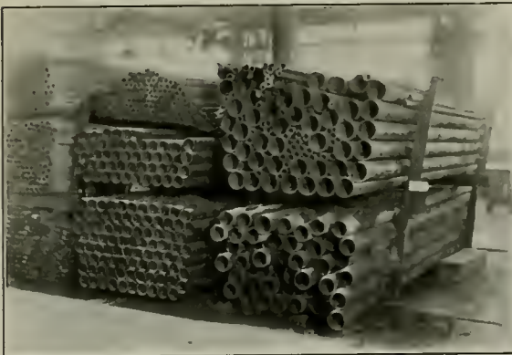
Fig. 2.—Tubes and Flues Stacked to Occupy Minimum Space
