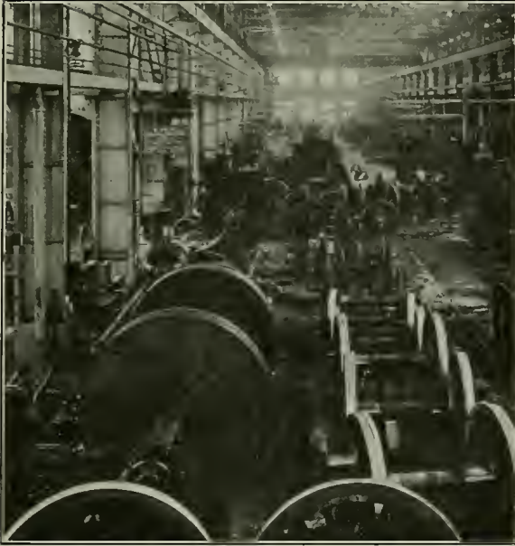
Driving Wheel Section of the Machine Shop Showing the Route of Wheels from and to the Erecting Shop
