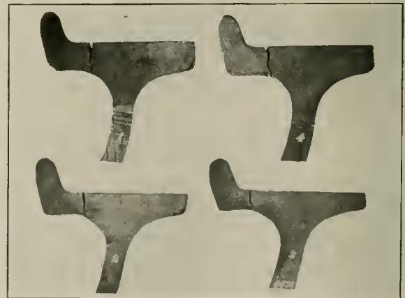
Fig. 6—Failures of 1-in. Sections Taken From Steel Wheels.
