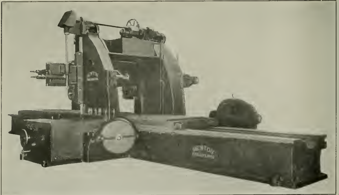
Fig. 2—View of Newton Horizontal Milling Machine from the Rear of the Operator's Side of the Table
