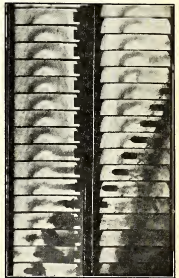
FILMS OF A BULLET FIRED FROM A REVOLVER; SHOT FIRED FROM A SHOT-GUN; AND A SHELL LEAVING THE MUZZLE OF A GUN. (FOR EXPLANATIONS SEE NEXT PAGE)
