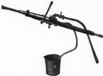
Sullivan Air Jet Drifting Stoper, with Water Spray
