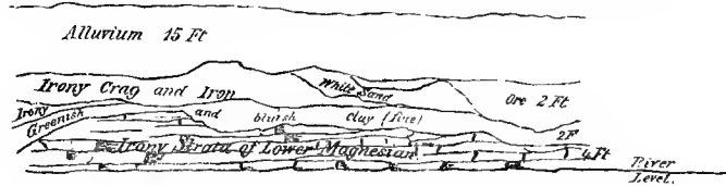
FIG. 26. SECTION IN THE BANK OF MAPLE RIVER, RAPIDAN.
