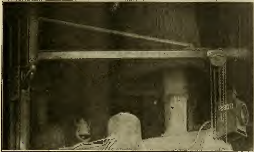
PERMANENT JIB CRANE ON OUTER LINE OF POSTS. ONE OF THESE CRANES BETWEEN EACH TWO PITS AT EAST ALTOONA ENGINE HOUSE—PENNSYLVANIA RAILROAD.
