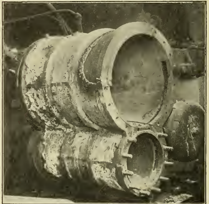
THE CYLINDER AFTER NEW PIECE WAS WELDED INTO PLACE
