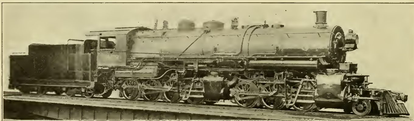
ARTICULATED LOCOMOTIVE OF THE 2-6-8-0 TYPE—GREAT NORTHERN RAILWAY.
