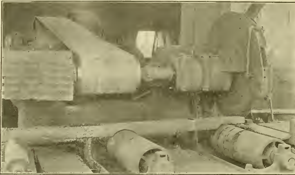
A BELT DRIVING A FRICTION SAW AND OPERATING SUCCESSFULLY IN EXCEPTIONALLY SEVERE SERVICE.
