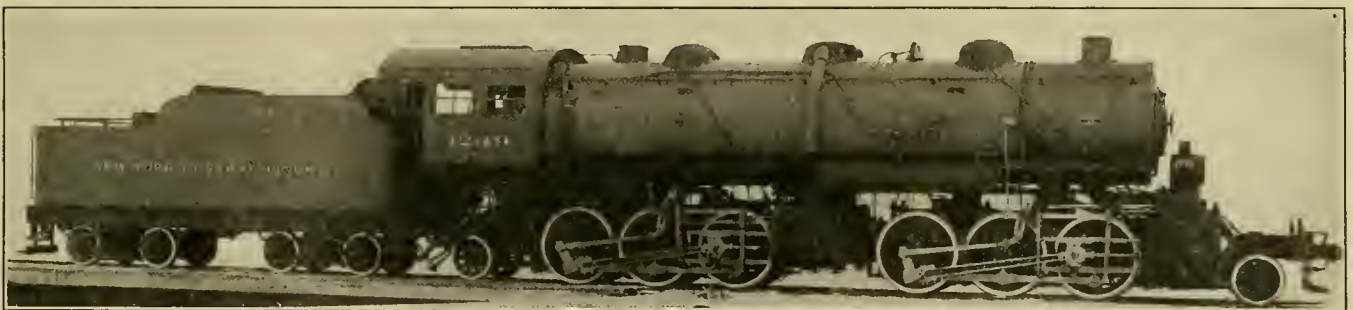
LARGE 2-6-6-2 TYPE LOCOMOTIVE BUILT FOR THE BOSTON AND ALBANY RAILROAD BY THE AMERICAN LOCOMOTIVE COMPANY. THIS IS THE FIRST EXAMPLE OF THE MALLET TYPE TO BE PUT INTO SERVICE ON THE NEW YORK CENTRAL LINES.
