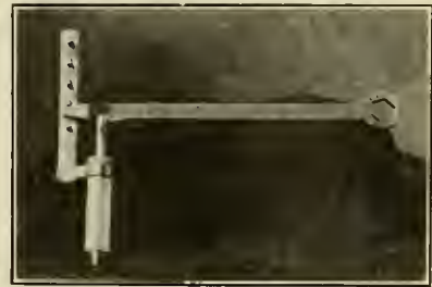
PUMP FOR FILLING RESERVOIR WITH GREASE.
