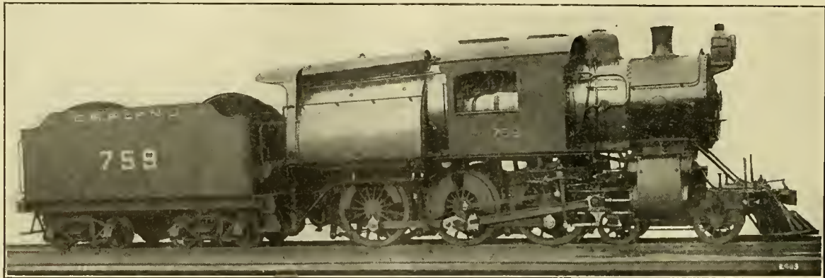
HIGH SPEED LOCOMOTIVE FITTED WITH THE IMPROVED BAKER-PILLIOD VALVE GEAR
