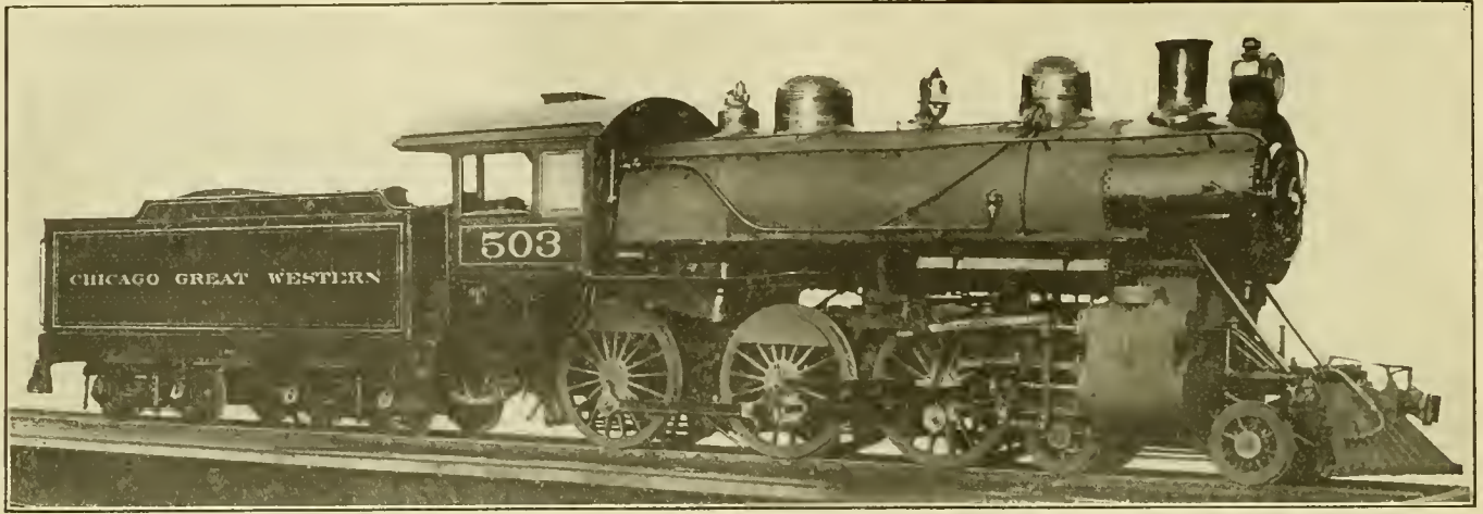
TEN-WHEEL PASSENGER LOCOMOTIVE WITH EMERSON SUPERHEATER—CHICAGO, GT. WESTERN RAILWAY.
