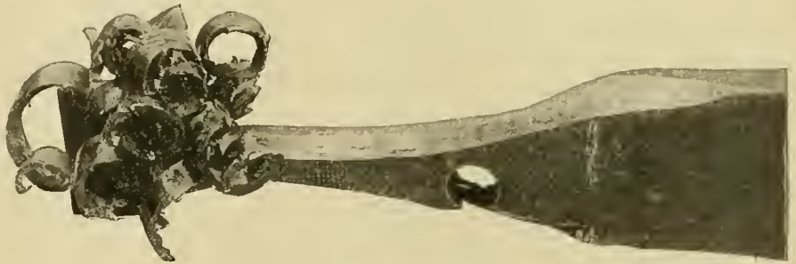
EXAMPLE OF WORK DONE BY A MECHANICALLY DRIVEN CHIPPING HAMMER.
