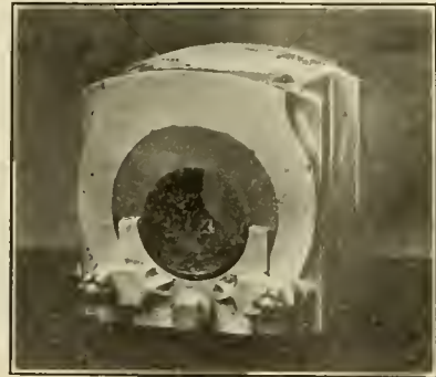
DRIVING BOX WITH REMOVABLE BRASS ASSEMBLED.
