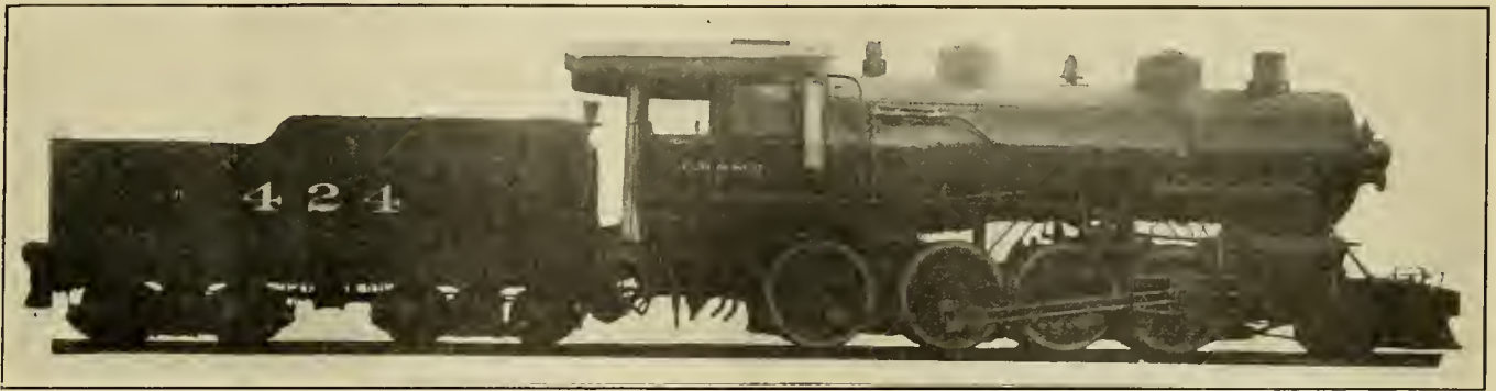
HEAVY CONSOLIDATION TYPE LOCOMOTIVE DESIGNED AND BUILT BY THE C. M. & ST. P. RY.
