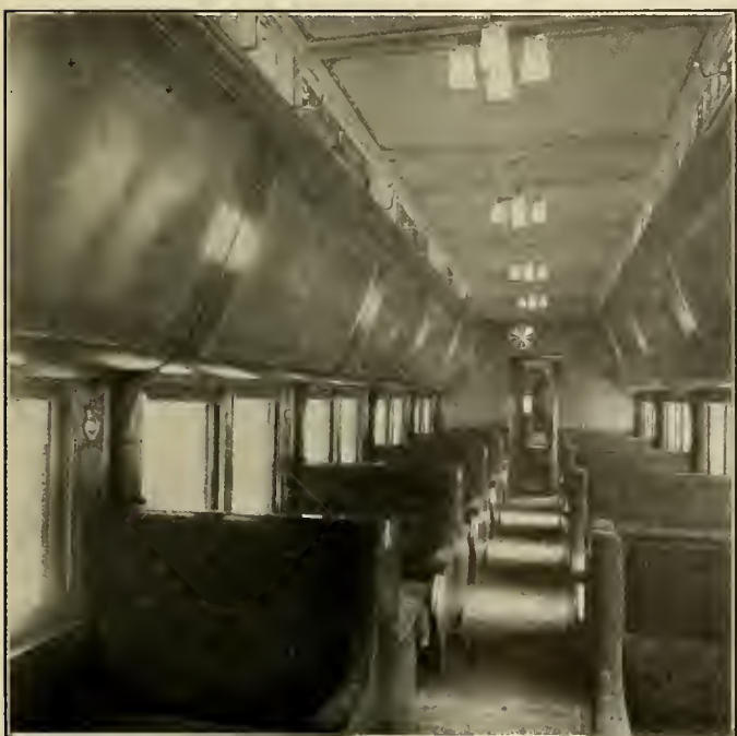
INTERIOR VIEW OF SLEEPING CAR. THE CEILING IS FLAT.
