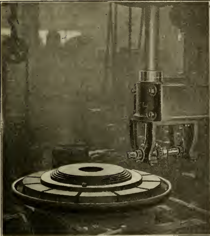
JIG FOR MILLING STEAM PORTS IN CYLINDER BUSHINGS. THE MILLING CUTTER HAS A VERTICAL ADJUSTMENT AND THE PLATE ON THE TABLE IS ARRANGED TO PERMIT THE QUICK AND EASY CLAMPING OF ALL SIZES OF BUSHINGS. THE CIRCULAR MOVEMENT OF THE TABLE IS AUTOMATIC AND THE PORTS ARE MILLED WITHOUT REQUIRING ANY DRILLING.
