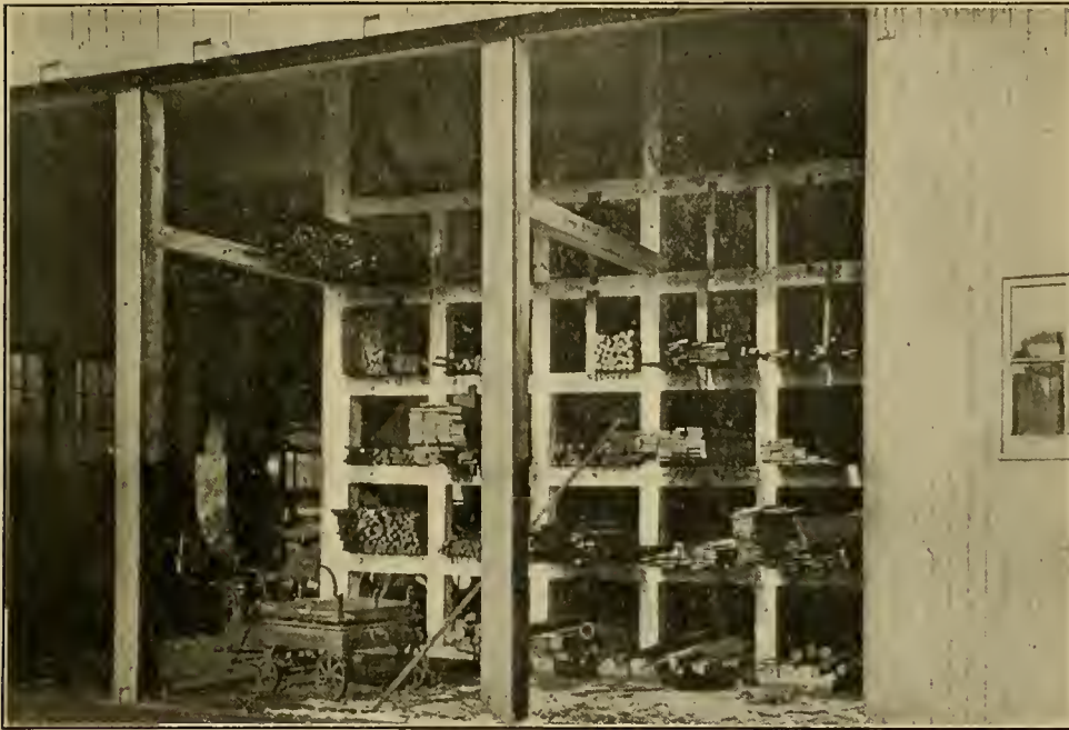
VIEW SHOWING THE IRON STOCK HOUSE LOCATED JUST OUTSIDE OF THE BLACKSMITH SHOP. THE SHEAR FOR CUTTING OFF THE STOCK IS SHOWN AT THE LEFT AND PORTABLE SCALES IN THE FOREGROUND. A COMPLETE STOCK OF BAR IRON IN COMMERCIAL SIZES IS MAINTAINED IN THIS BUILDING UNDER THE CHARGE OF A STOREHOUSE EMPLOYEE.
