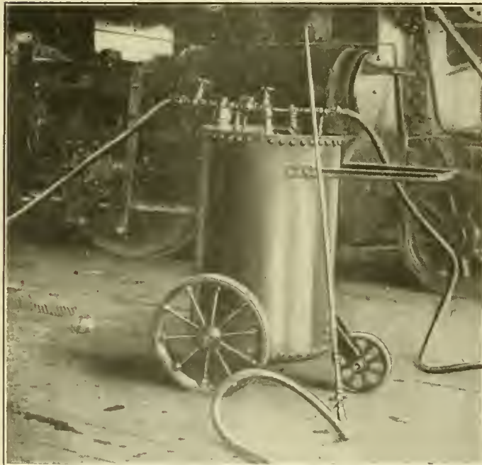
CRUDE OIL FIRING UP MACHINE, ASHTABULA ENGINE HOUSE—LAKE SHORE & MICHIGAN SOUTHERN RAILWAY.
