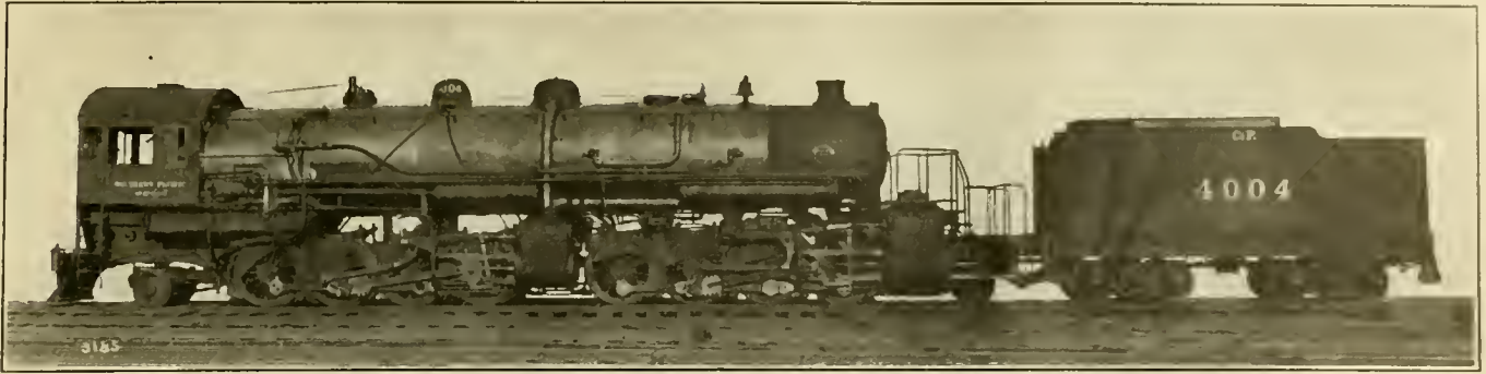
SOUTHERN PACIFIC ARTICULATED OIL BURNING LOCOMOTIVE WITH CAB AT FRONT END.
