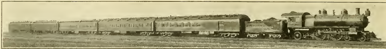
FIRST SOLID STEEL PASSENGER TRAIN, COMPOSED OF DAY COACHES, DINING CAR, AND PULLMANS, OPERATED BY THE PENNSYLVANIA RAILROAD COMPANY, AND THE FIRST SUCH TRAIN EVER OPERATED ANYWHERE.
