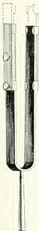
FIG. 471.—Dench's large tuning-fork with clamps at ends, giving 64 v. s., and without clamps 26 v. s.
