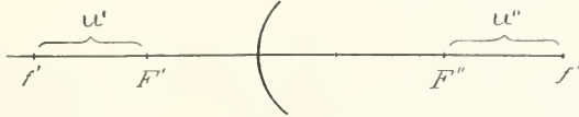
FIG. 63.—Showing the relation of conjugate foci to principal foci. Symmetrical notation about F' and F'' as origius.
