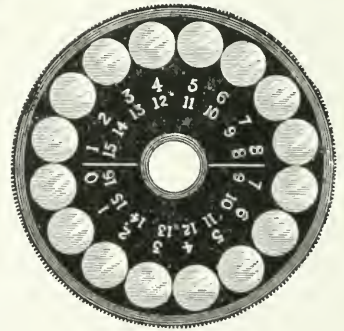
FIG. 118.—Loring's ophthalmoscope, with tilting mirror, complete disk of lenses from -1 to -8 and 0 to +7 , and supplemental quadrant containing +0.5 and +16 D. This affords 66 glasses or combinations from +23 to -21 D.
