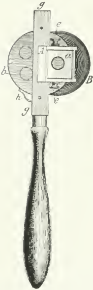
FIG. 117.—Ophthalmoscope of Helmholtz: the concave shade B is set at the side of the handle, a , with disks of lenses ( b ) centering at its sight-hole. In front of this a triangular case projects, carrying three thin glass plates at an angle of 56^\circ to the line of sight, by means of which the light is reflected into the observed eye.
