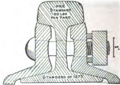
Fig. 121. ANGLE SPLICE BAR, PENNSYLVANIA RAILROAD, 1875. (From a drawing in the U. S. National Museum.)
