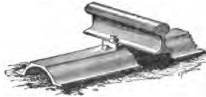
Fig. 105. METAL TRACK, GREAT CENTRAL RAILWAY OF BELGIUM, 1889. (From a drawing in the U. S. National Museum.)
