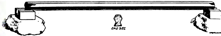
Fig. 25. WYATT'S HEXAGONAL RAIL, BANGOR, NORTH WALES. (1802.) (From model in the U. S. National Museum.)
