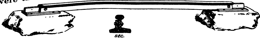
Fig. 24. EDGE RAILS, LAWSON COLLIERY, NEW CASTLE-ON-TYNE. (1797.) (From model in the U. S. National Museum.)
