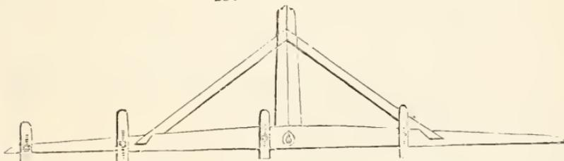
and for the purposes of road-making and irrigation it is furnished with plates of iron with adjusting screws, for the purpose of determining the slopes of surfaces.
