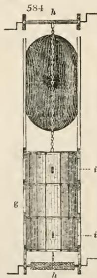
and bottom (fig. 583.), with doors to the fuel-chamber and ash-pit (fig. 581. c, d), and an arched cover to the top (fig. 584. g), which moves on small wheels, is drawn off
