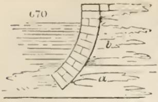
Caledonian Canal; and perhaps the finest in the world are the granite walls which embank the Neva at Petersburg, the construction of which may serve as an example of a river cased with stone on a foundation of soft bog earth.
