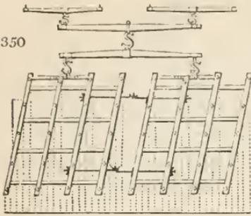
drawn at right angles to the line of the harrow's motion, shall divide the space between each bar into equal parts; so that the various teeth, when the instrument is moved forward, shall equally indent the surface of the ground over which they pass. (*Quart. Jour. Agr.*)
