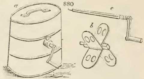
removed, the beaters (b) may be taken out at pleasure by withdrawing the spindle (c) to admit the removal of the butter, or the cleaning and scalding of the churn.
