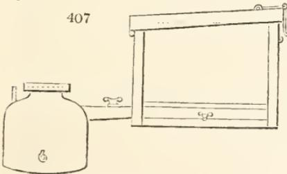
2805. *A steaming-machine, on a simple and economical plan* (fig. 407.), consists of a boiler, and wooden chest or box placed over or near it. The box may be of any size, and so placed as to be supplied and emptied by means of wheel or hand barrows in the easiest manner, either by the end or top, or both, being made to open. If the box is made eight feet by five, and three deep, it will hold as many potatoes as will feed fifty cows for twenty-four hours, and these may be
