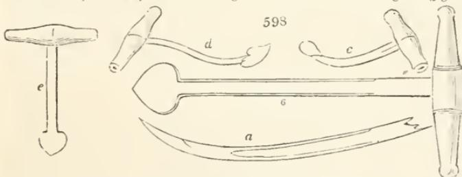
across the tree, in lengths of from two feet six inches to three feet. Having thus made the incision in the bark, both ways, the barkers being also each furnished with peeling irons of different sorts (b, c, d, e); if the tree or piece of timber to be barked is such as the two barkers can easily lift one end of it,
