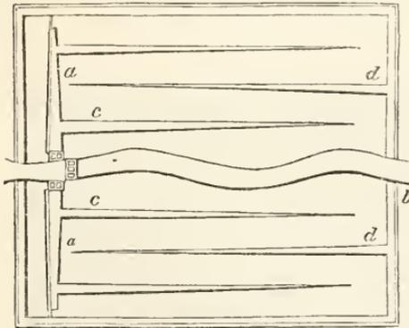
water flows along the highest part, or crowns of the ridges in the trenches (*c*), and is carried off to the tail drains by the trench drains (*d*).
