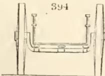
2767. *The Gloucestershire waggon*, according to Marshal, is the best in England. By means of a crooked side-rail, bending archwise over the hind wheel, the bodies or frames of them are kept low, without the diameter of the wheels being much lessened. The bodies are likewise made wide in proportion to their shallowness, and the wheels run six inches wider than those of most other waggons, whereby advantages in carrying top-
