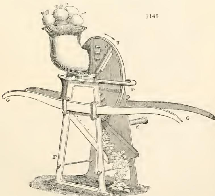
Scotland. It is made, when of full size, entirely of cast iron, and consists of a standard or frame to which is attached a hopper; the frame bearing a circular plate of cast iron mounted on a horizontal axis, to
