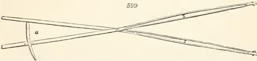
a brass limb or index (*a*), on which are engraven figures denoting the quarter girth in feet and inches. Raising the instrument, the index end (*a*) is taken hold of, and the other applied to that part of the trunk where the girth is to be taken, opening it so wide as just to touch. At the same time both sides of it, keeping the graduated index uppermost, on which the quarter girth will be shown, allowing one inch in thirteen
