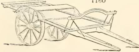
for the conveyance of timber, by simply unbolting the frame from the shafts, and in its place laying two single cross bars, one before, and another behind the wheels." (*Trans. H. S.*, vol. xi. p. 396.)
