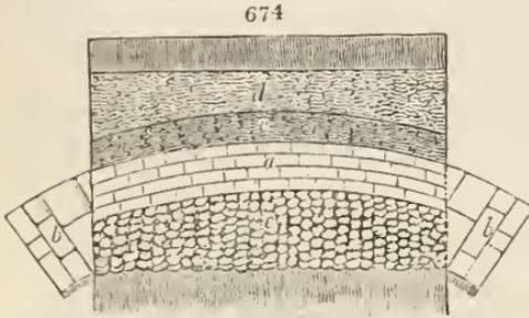
deepened for the purpose of drainage, so may their waters require to be raised for the purpose of irrigation, impelling machinery, or producing cascades or waterfalls for the purpose of ornament. Dams or weirs for this purpose should be constructed so as to form a segment of a circle across the bed of the stream, with the convex side pointing up the stream, and the ends abutting against a natural or artificial bank (fig. 674.) By this construction, the force of the
