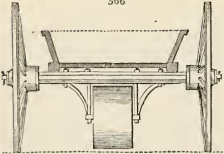
suggests the idea of placing a roller between the other wheels (fig. 566.), and so strongly secured to the axle tree, as to be able to support the whole weight in the cart when necessary. This roller he proposes to call a protector, and he thinks it will be much more easily drawn than two wheels running in deep ruts. (*Com. to B. of Ag. vol. i. p. 154.*)
