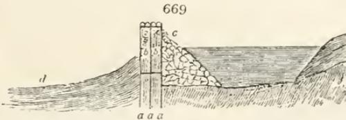
It consists of piles or poles, being the thinnings of plantation of Scotch pine and larch, driven six feet into the sand (*a a a*): the spaces between these piles (*b b*) are filled in with furze or other spray or small branches; and on the top of them, are wedged in stones to
