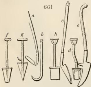
4309. *The draining shovel* (*d*) is another sort of implement employed for the same purpose as the above. It is made with a crooked handle, and the edge of the shovel part is turned up, in order to prevent the materials from falling off.
