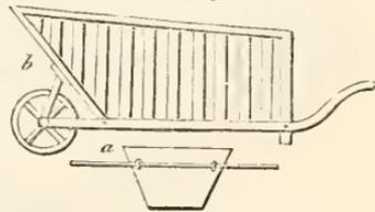
2540. *Barrows for hay and straw* may be variously constructed, and near towns (figs. 250, 251.) may be used for wheeling light packages.
