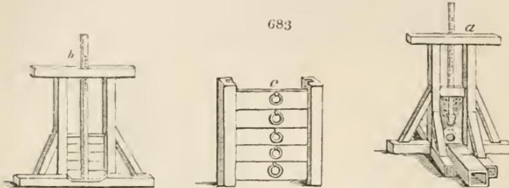
4407. *A trunk* is a covered sluice, being a necessary construction in all cases where two streams of water are to cross each other, to serve as a bridge for that stream which is to pass over or under the other.
