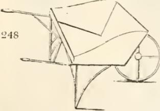
the latter (b) may be made to separate from the frame and wheel, and by means of levers (a) to be carried like the hand-barrow.
