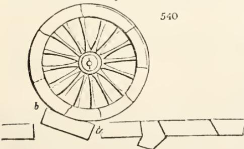
of the feet of animals, because the fulcrum (*fig. 540. a*), is continually changing its position: but if the stones of the road are large, then the wheel acts as a compound lever, raising up the one end (*b*), and depressing the other (*a*), of every stone it passes over; and in this case becomes more injurious on a bad road than the feet of loaded animals. The reiterated operation of this effect, by wheels following in the same track, soon destroys badly constructed roads.
