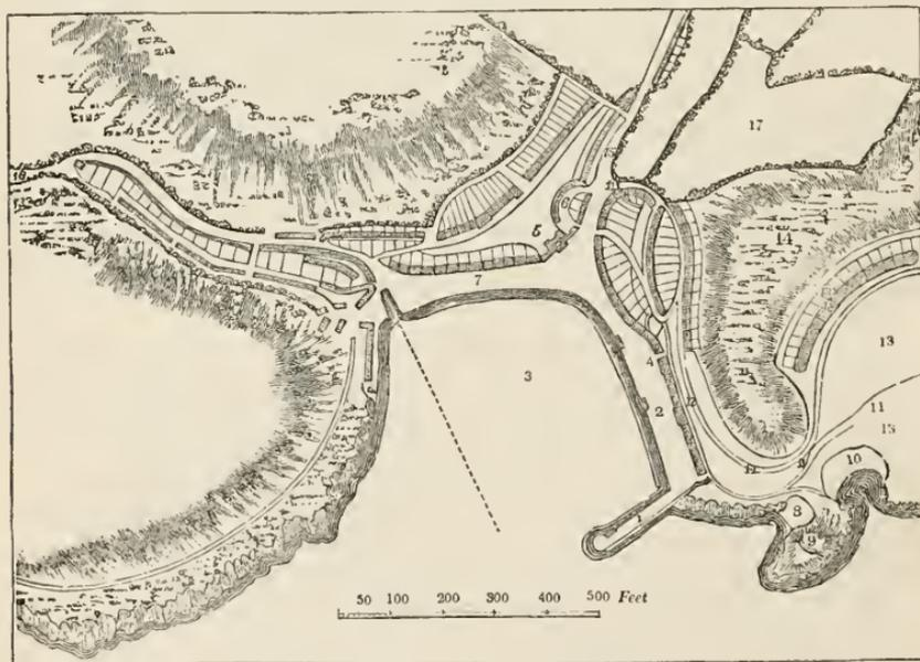
is given in the *Devon Survey*, and is described as containing a pier (1), quay (2), harbour (3), warehouses (4), inn and garden (5), stables (6), strand (7), cove for building ships and timber yard (8), beacon (9), cove for bathing machines (10), new carriage-way to the park (11), terrace (12), the park (13), plantation (14), road to Torwood (15), road from Newton, &c. (16), meadows (17), circus in the park (18).
