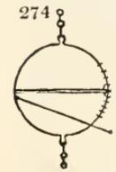
2565. *Braby's draught-machine* (fig. 275.), consists of two strong steel plates, joined at the ends, and forming a spheroidal opening between them. In using it, one end (a) is hooked on the muzzle of the plough or other implement,
