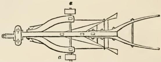
2641. Morton's draining plough (fig. 316.) has three coulters (a a b), two mould-boards (c c), and one share (d). The mould-boards have an inclined plane, formed upon
