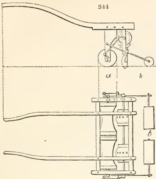
2687. Of *turnip drills*, the best, when this root is cultivated on a large scale, is the improved Northumberland drill. (fig. 344.) The roller (a) which goes before the seed has two concavities, and thus leaves the two ridgelets in the very best form for the seed; after these are sown, two light rollers (b b) follow and cover them. It is drawn by one horse, sows two rows at once, and seldom goes out of repair.
