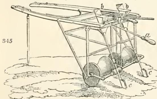
has two wheels which run in the hollows on each side of the drill or ridgelet to be sown;
