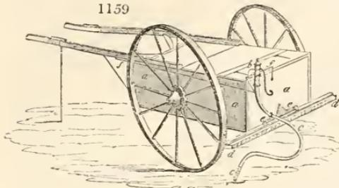
8195.—2711. *A cheap and useful water-cart* is thus described by Mr. Donaldson in the *Farmer's Magazine*, vol. viii., p. 81.:—A barrel, holding 160 to 200 gallons, is placed on a pair of wheels and shafts in the usual way. A pump, three inches in diameter, is placed close by the side of the
