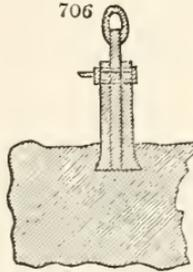
consists of a frame-work supporting a five-fold tackle, with blocks ten inches in diameter, and a roller seven inches in diameter turned by two long iron levers. A hole is made in the stone to be raised by means of the tool well known to masons as a *juniper*; in this hole a simple plug may be driven tightly; or a compound plug (fig. 706.) may be introduced; or, what is simplest, the hole may be made obliquely. (Smith's Compendium of Practical Inventions.)
