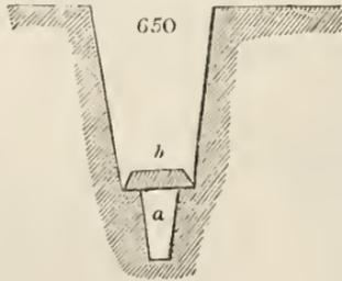
Where some sorts of moss, as Sphagnum or Lycopodium, can be got, these drains are of unknown durability. Drains formed in this manner, through tough and retentive clays, will be found, in a short time after the work is finished, to have formed over the straw with which the drain was filled, an arch of sufficient strength to support the incumbent weight of the soil and the casual traffic of the field. In twelve or
