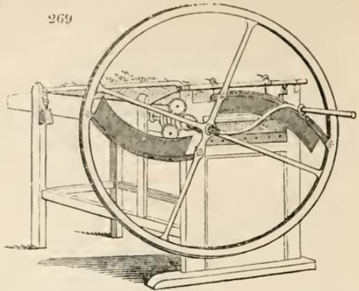
2561. *The hay-binding machine* is an invention by Beckway for weighing and binding straw or hay. (*fig. 272.*) It is a very ingenious apparatus, and may be useful to retail
