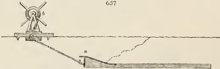
commencing at its lowest level, so as to work up hill. A windlass (b) is next placed at the full length of the rope, which is attached to the slide. Clay is next rammed firmly down on the slide with a heavy rammer to the depth of three or four inches, and the slide is next pulled forward, leaving a cylindrical drain of three or four inches in diameter, according to the diameter of the slide. (*Trans. Soc. Arts*, vol. xlvii. p. 20.)
