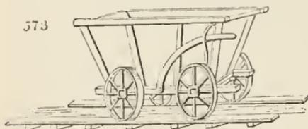
point as to be in danger of too much crushing the road; the carriages can be made much more limber and light in all their parts (*fig. 573.*), and they are much more easily moved, and more manageable in all respects, than they otherwise would have been. And another advantage of this arrangement, which deserves to be particularly adverted to, is, that it admits
