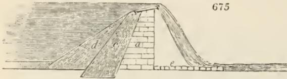
matter of any kind to a considerable slope (d). Beneath the dam a considerable portion ought to be paved (e). (*Gen. Rep. Scot.* vol. ii. p. 669.)
