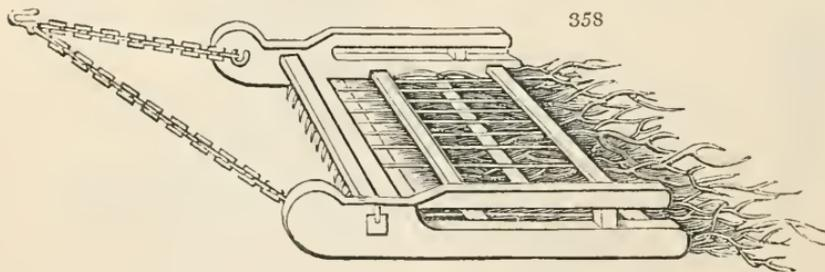
three or more cross bars, fixed into two end-pieces in such a manner as to be very rough and bushy underneath. To the extremities of the frame before are sometimes attached two wheels, about twelve inches in diameter, upon which it moves; sometimes, however, wheels are not employed, but the whole rough surface is applied to, and dragged on, the ground.
