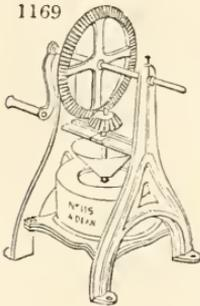
8210. *Brick and tile making machines* have recently been invented by various persons. One by the Marquis of Tweeddale is in most general use, and he has recently invented a hand drain-tile making machine, which was honoured with a premium in 1843. Messrs. Ransome have also brought forward a new machine for making tiles and bricks, which received a silver medal at the meeting of the *English Agricultural Society* at Derby in 1843.
