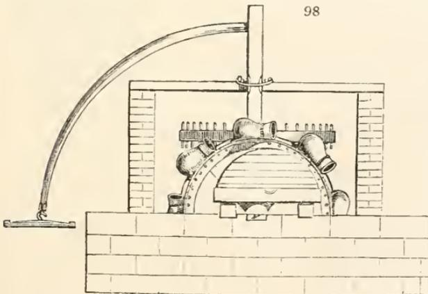
over a well has a series of earthen jars, fastened together by cords of esparto, which descend into the water and fill themselves ; by the motion of the wheel they
