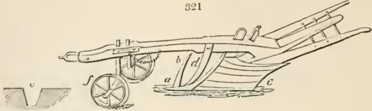
share (a) has a coulter (b) fixed to it, projecting upwards, to cut one side of the drain, and another coulter (d) fixed to the beam and also to the share at its lowest end. The turf which is thus cut out passes between the coulter (d) and the mould-board (e), and is thus lifted clearly out of the trench. The depth of the drain is regulated by the wheels at the fore end of the beam (f). This plough is drawn by four or six horses.
