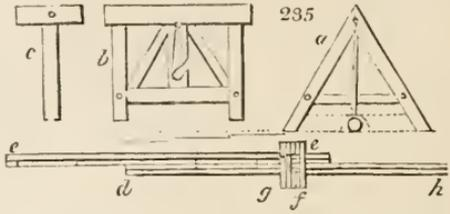
2503. *The object staff* (fig. 235. c) is used with the water or square level: for either it should be exactly of the same height as the level; the cross piece at top should be a foot or more in length, and three inches broad, painted white on one side for opposing to dark objects, and black on the other for opposing to such as are white.
