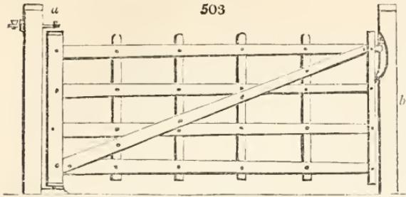
at proper distances between the middle and the head of the gate: these cross bars must, he thinks, assist very much in keeping the gate together; but what is most to be guarded against is its sinking at the head, to prevent which this gate is, he says, well contrived.
