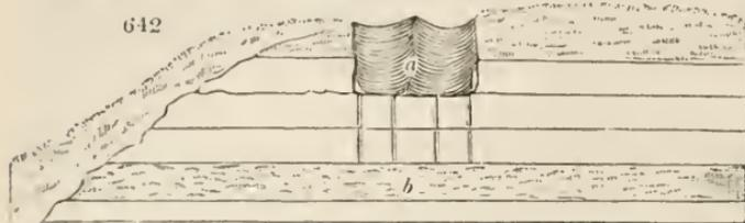
of rock or gravel, it may sometimes be drained by boring into the latter (b). In this way different chalk pits and lime quarries have been
