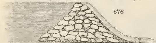
running rivers not subject to high floods, and where there is such a superabundance of water that no loss is sustained by the quantity which flows through the stones. Where it is required to retain the whole of the water, a puddle bank should be carried up the middle of the dam. (*Ibid.*)
