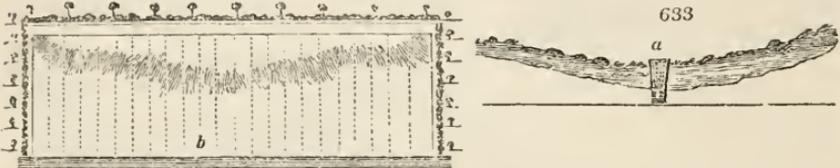
to that depth through the middle of the field, if it have a descent from both sides; but if it decline all to one side, the drain must be made on that side (b), as the water will more readily discharge itself into it; and, unless the field be of great extent, and have more than one depression or hollow in it, one drain may be quite sufficient for the purpose, as by crossing the different beds that retain the water, it must take it off from each.
