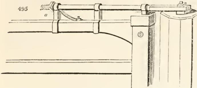
to their falling; all that is necessary, when the gate sinks at the head, is to screw it up by the nut (a) till it regains its original position. For road and farm-yard gates the hinges are valuable parts of the construction.
