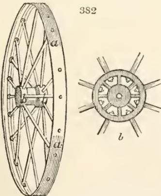
2750. *Jones's improved iron wheels* (*fig. 382.*) are formed wholly of cast and wrought iron. The felly, or periphery of the wheel (*a*), is made of cast iron, with conical holes on the outside, contracting towards the centre, through which the spokes, made of iron rods, are to be passed, and secured in the box, or nave (*b*), near the centre of the wheel, by nuts screwed on to the reverse end of the rods, by which means they are drawn tight. (*Newton's Journal, vol. i. 2d Series, p. 154.*)
