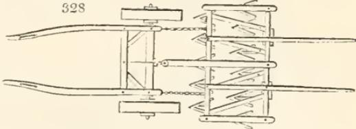
*are intended to pierce about two inches at each operation; so that by repeatedly passing it over the surface, the land will be stirred deep as the plough has gone.*
