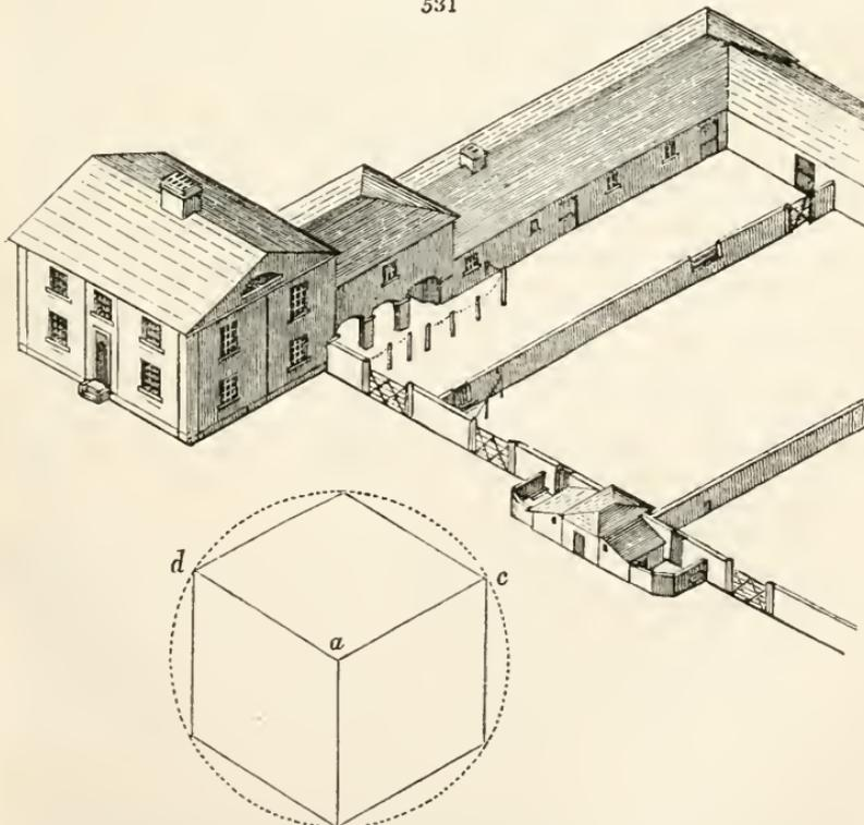
made in rays parallel to the diagonal of a cube upon a plane perpendicular thereto. This is a comprehensive and useful method of exhibiting the several parts of a homestead, and any person moderately acquainted with drawing, if they make the attempt, will find it extremely easy to perform; nothing more
