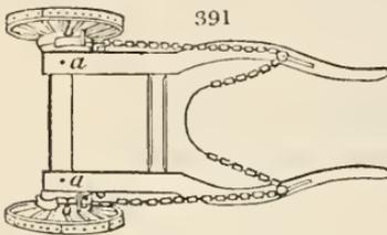
apparatus, exhibiting the framing of the cart, the shafts, wheels, and brakes; the chains also are shown, passing from the bars on each side, each round a horizontal pulley on the shaft, and attached to the ends of the breeching. Thus it is evident that, when a cart, furnished with this drag, is going down hill, the load, pressing the breeching against the horses, draws the brake tight by means of the chain, and produces a friction on the nave proportioned, in some measure,
