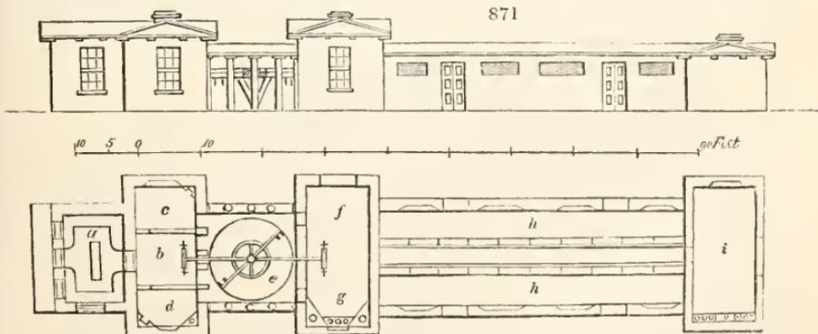
hollow walls, double doors, double sashed windows, and an ice-house under. The milk room (*a*) is surrounded by milk coolers, and has a butter slab and jet in the centre. The jet is supplied from a cistern over the steaming house (*f, g*), to which the water is raised from a well by a forcing-pump worked by the
