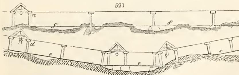
line be straight or curved in direction, can only be determined on an irregular surface by measuring down from an elevated level line (a), or from level lines in parallel directions,
