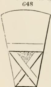
4290. The spray drain is generally, like the gravel drain, of small size, and formed, like it, with an acute-angled bottom. In general, the spray is trowed firmly in; though in some cases it is previously formed into a cable, as in the brush-wood drain. Drains of this sort are much in use in grass lands, and when the spray of larch wood,
