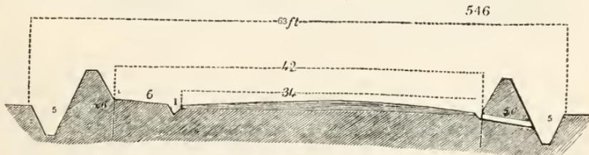
3679. *The degree of convexity preferred by Walker* is just a sufficient rise towards the middle, to incline the water to the sides; and in place of making the whole width the section of one curve, to form it by two straight lines, forming inclined planes, and joined by a curve towards the middle. "I have seen," he says, "ridges formed in what I
