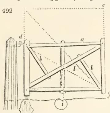
The half of the right angle (c e g) seems a reasonable limit, by which, if the power requisite to hold the weight in equilibrium, when acting at a right angle, be as the side of a square of the length of the lower bar of the gate (g c), then the power requisite to effect the same end, when acting at an angle of 45 degrees, is as the diagonal to this square (g h). By changing the square to a parallelogram, the rela-
