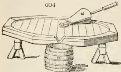
4144. *An eligible description of mill*, where cider is only made for private use, consists of a pair of fluted rollers working into each other. These rollers are of cast-iron, hollow, about nine inches in diameter, with flutes or teeth, about an inch wide, and nearly as much deep. In general they are worked by hand, two men working against each other. Between these the fruit passes twice; the rollers being first set wide to break it into fragments, and afterwards closer to reduce
