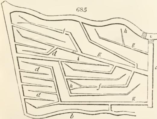
is a sluice (*i*) erected at the end of one of the small mains, to force the water into the branch trench adjoining (*f*), that being the highest ground.
