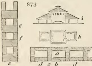
feet wall. The passages communicate with the roof by covered openings, in the ridge of which and by the windows ventilation is completely effected. In detail, the plan exhibits two principal entrance porches (*a*), back entrance (*b*), copper for heating water (*c*), churning-room (*d*), milk-room (*e*), utensils
