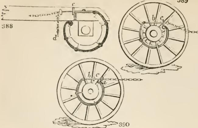
pieces of wood, "united on the outside by a strong jointed iron hoop; the wood pressing upon the nave of the wheel. The first, a fixed pivot (a), from the hoop, is fixed to the under side of the frame of the cart; from the other extremity of the hoop of the brake proceeds a bar (b), which slides through the plate or socket (c) fixed
