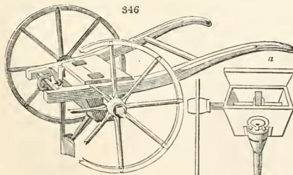
2689. *The Northumberland one-row turnip drill* (fig. 346.) by which means the sower is enabled to keep the row exactly in the centre of the drill. The ridgelets are previously rolled, either by a common or concave roller; the latter being preferable: and as the horse goes in the furrow at one side of the drill to be sown, of course he draws from one side of the draught-bar of the barrow. A small roller follows, and covers and presses in the seed. A recent improvement in this machine
