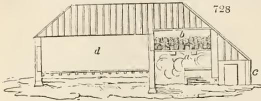
5143. *The kiln* (fig. 728.) in general and established use throughout Russia, for the purpose of drying corn in the straw, is heated commonly by fires of wood. It is a simple and cheaply erected structure, the walls eight feet high, and fifteen feet square within. At this height there are two strong cross-beams (a), to support the small timbers, laid over them as ribs. The corn stands in sheaves above these ribs (b), closely set up, the band ends of the sheaves down,
