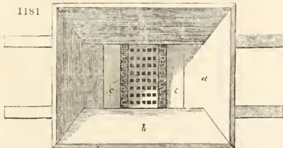
in length, and is moved by the crank handle (*d* in fig. 1182.); *c* c are two wedge-shaped pieces of hard wood,
