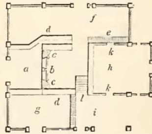
the cattle, and is thus kept always dry (k); door and staircase leading up to the wool chamber (l). The stairs rise quick, so as to be quite out of the way of the ox feeding in that side of the house.
