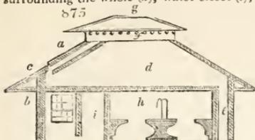
7004. A section (fig. 875.) taken across the milk-room (fig. 874 *n n*) exhibits the ventilating funnel in the roof (*a*), projecting eaves (*b, c*), cheese-room (*d*), passage on the north side (*e*), raised part of the roof for ventilation (*f, g*), fountain in the centre of the dairy (*h*), and south passage (*i*).
