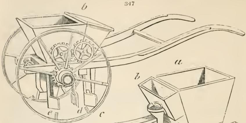
which forms the gutter for the seed (*e*). The seed is thus deposited about one inch above the manure. One roller of the concave kind goes before the machine, and another light one of the common kind follows after it: or, without attached rollers, the drill may be affixed to one side of the common roller behind, which roller may prepare one drill and cover the seed sown on another each course.
