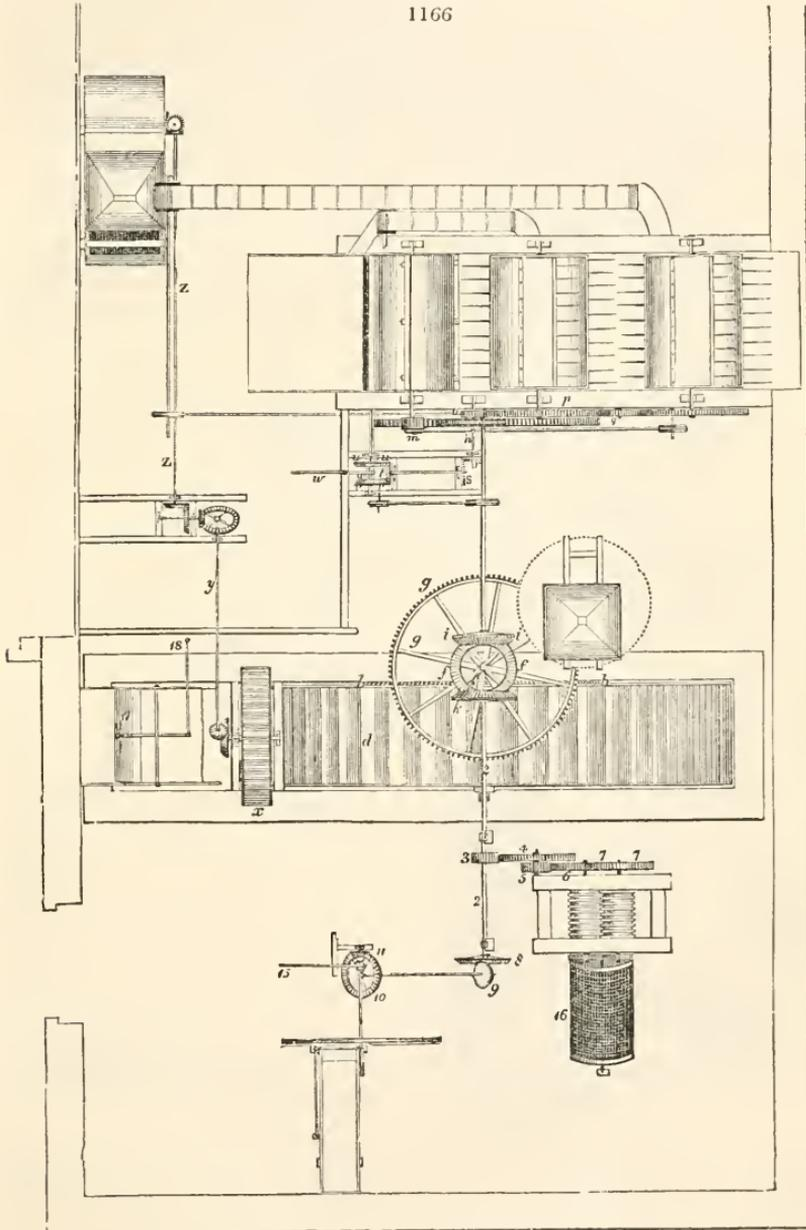
On the shaft 2 is a bevel wheel, 8, of 46 cogs (twenty-one inches diameter), driving the pinion 9, of 16 cogs (nine inches diameter), on an inclined shaft leading to the floor above; on the upper end of this shaft is a bevel wheel, 10, of 52 cogs (twenty inches diameter), driving a pinion, 11, of 17 cogs (nine inches diameter), on the spindle of the chaff-cutting machine.
