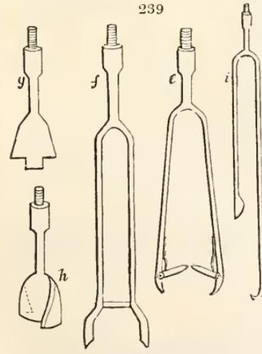
2514. *The chisel or punch-pine (g)* has a projecting piece to be used for penetrating through stone. This chisel is by rising and falling made to peck the stone and pulverise it, the small middle part breaking it away first, and afterwards the broad part coming into action. Another chisel, or punching-tool (h), is twisted on its cutting edge, and is used for breaking away a greater portion of the stone.
