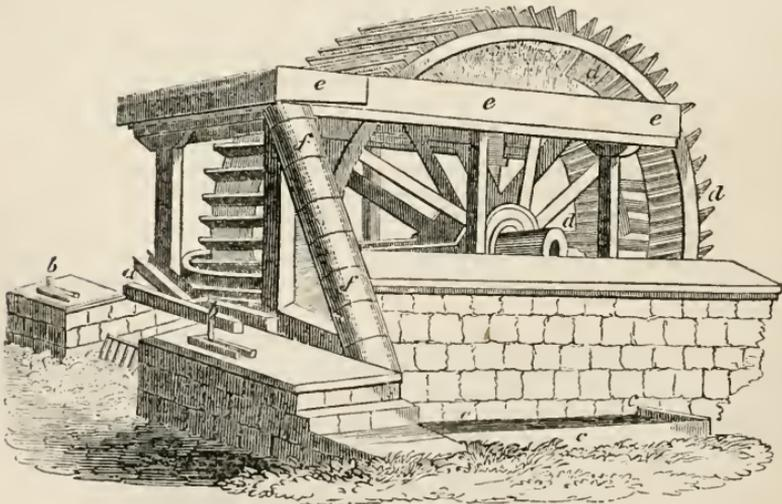
esting account in the *Farmer's Magazine*, vol. xviii, from which the present is extracted. Fig. 204. *a*, is a sluice through which is admitted the water that moves the wheel; *b b*, two sluices through which is admitted the water raised by the wheel; *c c c*, a part of one of two wooden troughs and an aperture in the
