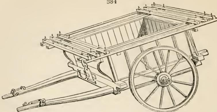
the cart. On drawing out an iron pin, the fore part of the body rises up from the shafts, while the other end sinks, and allows the load, whether of dung, earth, or stones in the close cart, or of hay, or sheaves of corn, on the cart and frame, to fall to the ground.
