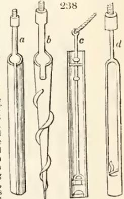
When this cylinder is lowered to the bottom of the bore, the bucket is lifted up by the rod and cord, and descends again by its own gravity, opening upwards like other lift pumps, which at every stroke raises a quantity of water and sand in the cylinder equal to the stroke, the ascent and descent of the bucket being limited by a guide-piece at the top of the cylinder, and two small nobs upon the rod, which stop against the cross-guide.
