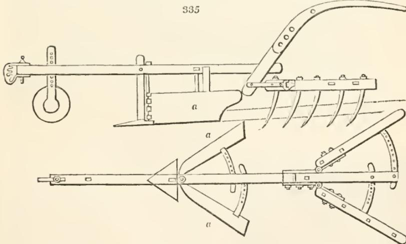
set to different distances, as it may be required, within the limits of twelve and thirty inches. The harrow which is attached to it is found advantageous in clearing lands from successive crops of weeds, as well as in bringing them to a proper state for the purpose of cropping; serving in this respect as a cultivator.
