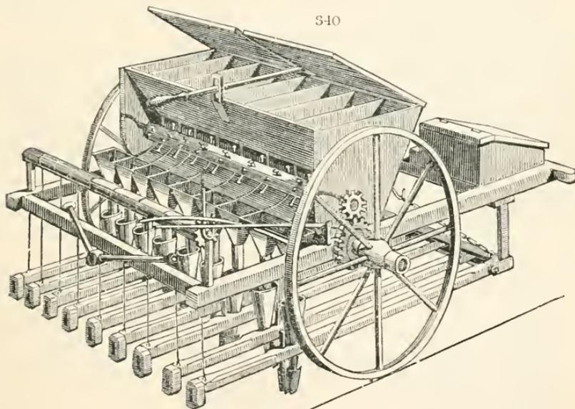
2681. *Cooke's three-row corn drill* is the large machine in a diminutive form, and is exceedingly convenient for small demesne farms where great neatness is attended to. It can be used as a cultivator, hoe, rake, &c., like the other.
