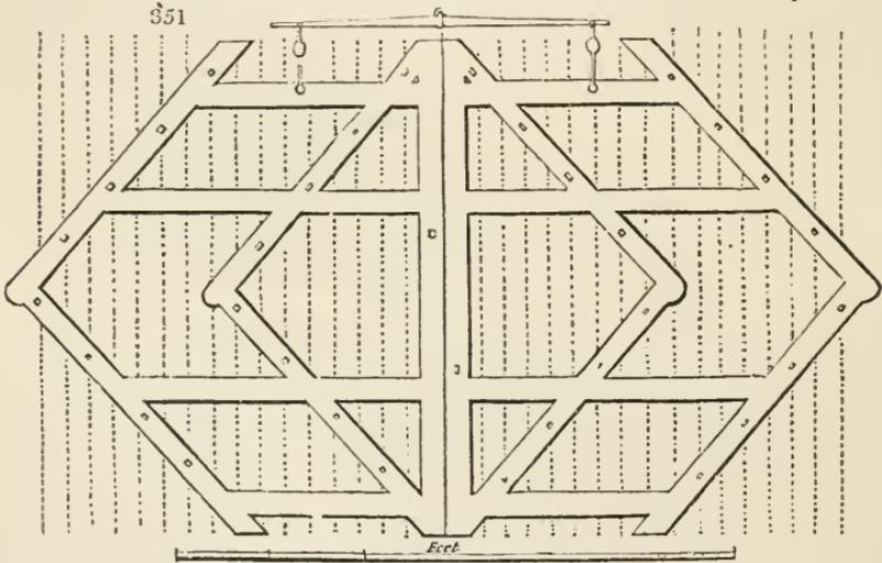
the kind, as it both operates on the ground with great regularity, and is less liable to ride or be deranged in turning, than the common, or the rhomboidal harrow.
