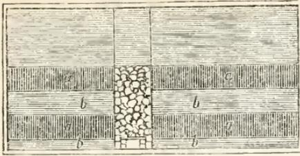
taining water; for in this case it is generally desirable to raise the stones above the level of the bottom of the upper seam, so as to convey away any water which may remain in it, to the conduit beneath (*fig. 637. a*, sand or gravel; *b*, clay); and it was a circumstance very generally observed in the course of operations, that where the upper stratum containing water was only a few feet in depth or thickness, another open stratum was generally found a few feet deeper.
