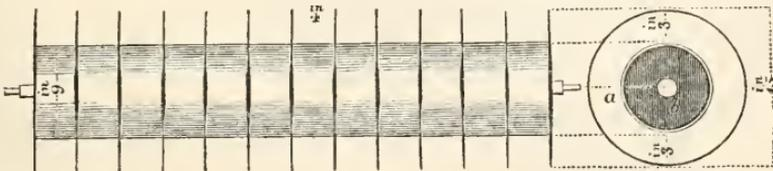
inches in thickness, and nine inches in diameter, and bound round with iron. Both blocks (a) and plates (b) are movable on an iron axle; and though Mr. Bartlett, the inventor, has adopted a diameter of nine inches for the blocks, and fifteen inches for the plates, yet these dimensions may be increased or diminished at pleasure. The frame in which the roller is inserted has a bar, on which are fixed scrapers of iron, which keep the roller continually clean. (Gard. Mag. vol. v.)
