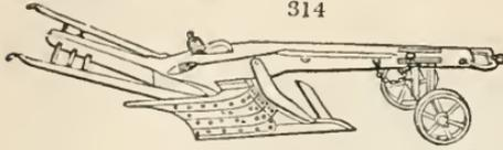
2640. Gray's draining plough (fig. 315.) seems one of the best. The beam is strongly fortified with iron, and is always kept at a proper distance from the surface of the ground, and also the
