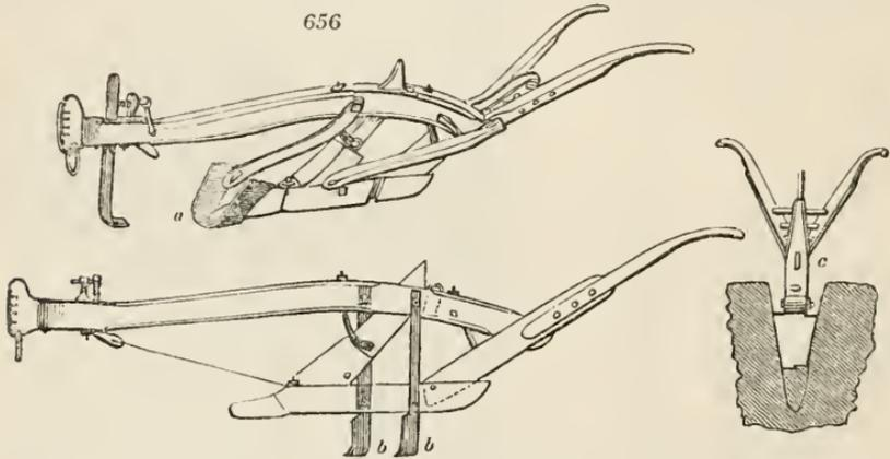
scoops. (figs. 653, c, and 651. a, b.) A second pair of coulters cuts the soil to the depth required, which is also taken out by the scoops. The total depth is now about twenty-six inches, the width at top ten inches, and at bottom about one inch. A slide (fig. 657, a) is then dropped to the bottom of the drain,
