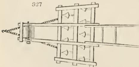
all the weed roots that lurk in the soil. Beans and peas have been sown in spring on the winter furrow, after being stirred by the grubber; and barley also after turnips, without any ploughing at all. This implement is made of different sizes, and may be worked either by four or by two horses, and one man.
