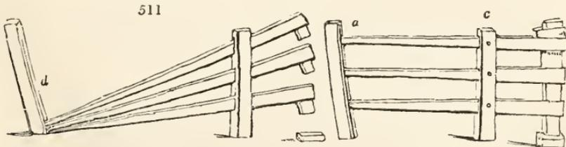
it consists of bars, light at one end (*a*) and heavy at the other (*b*), with concealed joints or pivots, in an upright post (*c*) placed nearer one end of the bars than the other. Then, while the weight of the short ends of the bars keeps them in a fencible position, a slight pressure on the other end will form a passage (*d*) which any one may easily step across.
