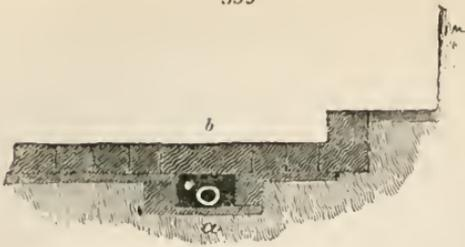
of flag-stones or cast-iron plates on a bed of mortar. (*fig. 559.*) When this mode is adopted in the streets of cities, the gas and water pipes (*a*) may be placed in drains, covered with large blocks of granite (*b*), channelled on the surface to prevent horses from slipping. Access to the pipes might be had by simply lifting these stones, without disturbing any other part of the pavement. (*Gard. Mag.* vol. v. p. 79.)
