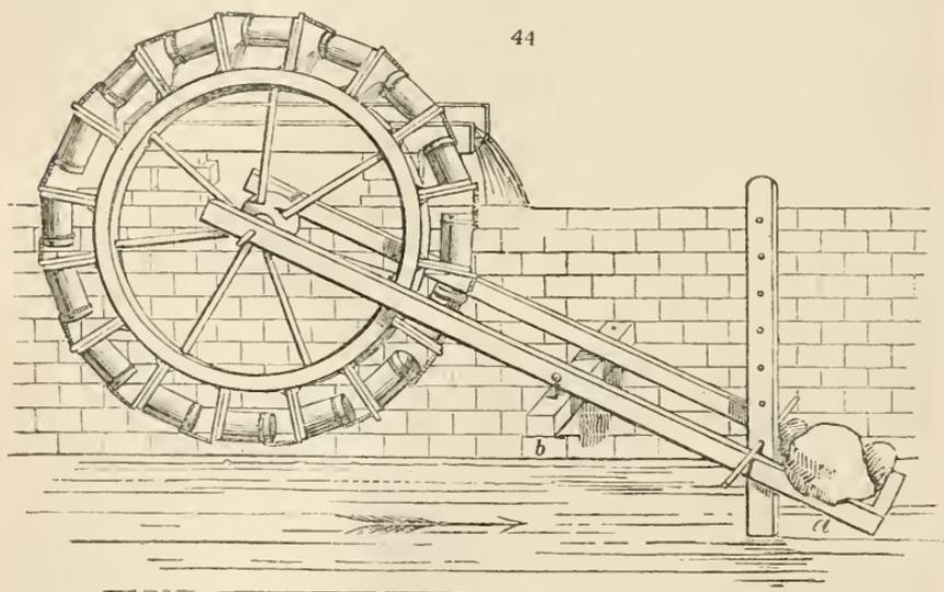
*Alps.* This wheel is raised or lowered by means of a loaded lever (*a*), which turns on a fulcrum (*b*), formed by a piece of wood with its end inserted in the river's bank.
