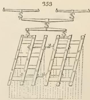
2700. *The common brake* (fig. 353.) is merely a harrow of the common kind, of
