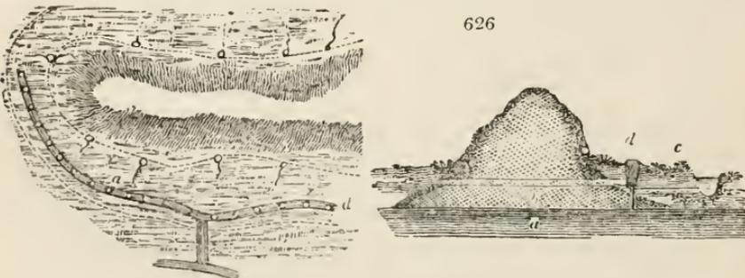
through a hill or rising bank, the surface of the low lands will, in general, be spongy, wet, and covered with rushes on every side (*c*). In this case, which is not unfrequent, a ditch or drain (*d*), properly cut on one side of the hill or rising ground, may remove
