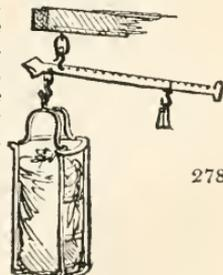
2569. *A potato-weighing machine* (fig. 279.), of a very complete description, has been invented by Mr. John Smith, of Edinburgh, and is figured in the *Highland Society's Transactions*, vol. vii. pl. iii. It is on the principle of the steelyard, and chiefly intended for weighing grain, flour, potatoes, or any other commodity usually put into a bag for carriage or keep. The machine is portable, of easy use, and not liable to go out of order.
