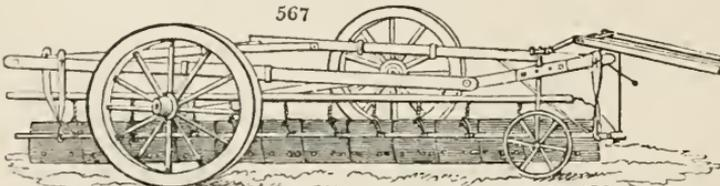
3749. *The scraping machine* (fig. 567.) is the invention of John Boase, Esq., and consists of an oblong frame of iron, supported on three wheels, two of which are common carriage-wheels, about three feet in diameter, working on an axle fixed to the frame; the third is a small cast-iron one, placed under the centre of the front bar of the frame. Below the frame, and obliquely to it, is placed the flexible scraper,
