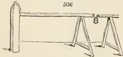
3101. The tressel-bar gate (fig. 506.) consists of two bars, one hung by a few links to each gate-post, and in the middle of the opening, where the bars meet, they are supported by two legs, like a tressel, and may be padlocked, or fastened by a pin and a few links, &c. In the promenade at Florence such gates are made use of to close the larger carriage openings.
