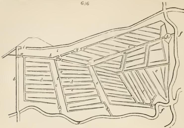
surface is formed into ridges (c, c), over which the water flows, and is carried off by the drains in their furrows (d, d), to the main drains (e, e), and to the brook at different places (f, f). There are bridges (g, g) over the main feeders, small arches over the main discharging drains (h, h), and three hatches (i, i).
