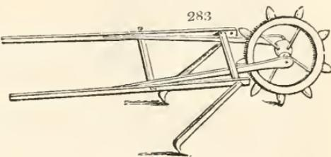
2575. *The common hand drill-barrow* (fig. 284.) consists of a frame and wheel somewhat similar to that of a common barrow, with a hopper attached to contain the seed. It is used for the purpose of sowing horse-beans, turnips, and similar seeds, upon small ridges. In using it, the labourer for the most part wheels it before him, the seed being afterwards covered by means of a slight harrow, or sometimes by a shallow furrow.
