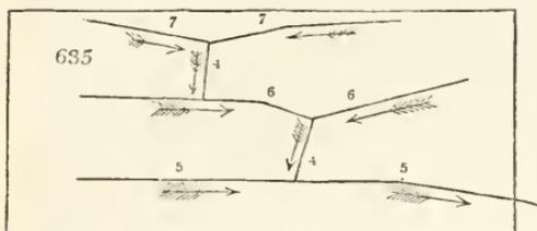
hole, in the line of the drain." The drains were next dug out, and formed ; some of them three feet wide at the top, six feet deep, and two feet wide at bottom, and others of different widths and depths, but generally in the same proportion. The following are Mr. Stephens's directions for building :—
