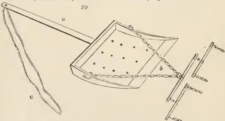
508. *The mouldebaert* (fig. 59.) is a curious and useful implement. It resembles a large square malt or cinder shovel, strongly prepared with iron on the cutting edge, and
