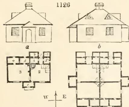
Each of such cottages is surrounded by a neat garden, containing a pisty, pump, and bee-house; and the house containing a porch (1), kitchen, oven, and stairs to bed-rooms (2), store (3), store closet (4), bed closet (5), pantry (6), coal closet (7), back entrance (8), tool house (9), and water closet (10), with two garret bed-rooms over.
