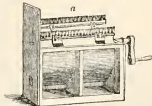
2553. The *furze-bruiser* (fig. 263.) is an ingenious and most useful machine where furze is either grown or found naturally. The shoots are bruised and cut into short lengths by hammers which operate like those in the mills for hammering iron. When the material is not sufficiently bruised, it is afterwards passed between rollers.
