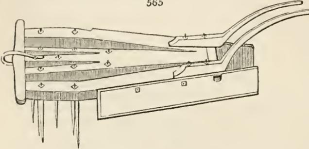
3745. *Harriott's road harrow* (fig. 565.) has been used in some places, for dragging over roads when much out of repair, to replace the stones or gravel disturbed by wheel carriages. "A man, a boy, and two horses, will do three miles in length in one day; completely harrowing down the quarters, and drawing the stones together, which, by means of the mould-boards, are dropped into the ruts far better than a man can stub them in."
