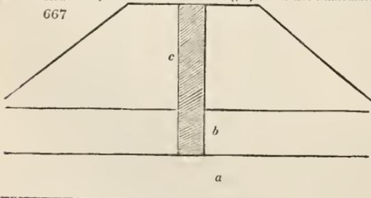
pinned down, or the new turfs rendered by some other means not easily softened and raised up by the water, will end in a breach of the bank. A similar effect is produced by a surface formed of unequal degrees of hardness and durability. The banks of this description in Holland, at Cuxhaven, and along the coast of Lincolnshire, are regularly watched throughout the year; the surface protection is repaired whenever it goes out of repair; as is the body of the bank in the summer season.
