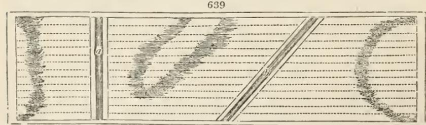
the ridges and furrows formed accordingly, may be sufficient for effecting its drainage. There may, however, be cases, as where a field is large and very flat, in which some side-cuts from the principal drain may be necessary, which must be made a little into the clay, and as narrow as they can be wrought, and then filled up with stones or other suitable materials.
