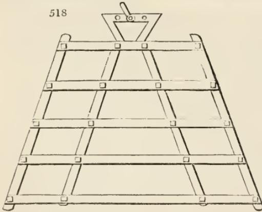
than when a smaller number is employed: the improved forms, calculated to cover the breadth of two or more of the old harrows by one frame (*fig. 518.*), are only calculated for flat ridges, or for working dry lands in which ridging is not requisite.
