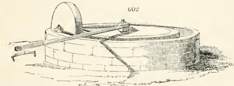
is sometimes divided into compartments for containing different varieties of the same fruit. (*fig. 603.*) The size of the runner varies from two and a half to four
