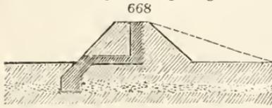
puddle wall from the retentive stratum. Such was the difficulty in some cases, that the puddle could not be carried up perpendicularly, but a puddle wall being raised within the bank, as high as the natural surface, it was joined horizontally to another puddle wall in the body of the bank. (fig. 668.)
