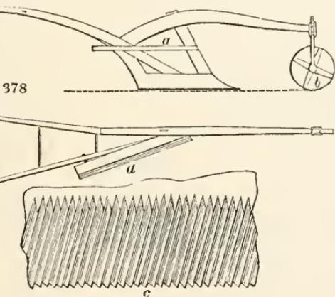
of Scotland with complete success. The framework of this machine is the same as that of a common plough. To this is added the knife (*a*), which is a plate of steel, screwed to a piece of wood, to keep it from bending up and down; this wood being screwed to the framework. There is a wheel (*b*) to keep the knife when in motion in a horizontal position. The cutting edge of the knife (*c*) has teeth, or serrations, on the upper side (*d*); the under side (*e*) is flat.
