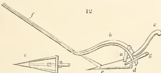
In it we have the other parts, the aura or mould board, and the coulter, composed no part of the simplest form of Roman plough; the plough-staff, or paddle, was a detached part; and the manicura, or part which the ploughman took hold of, was a short bar fixed across, or into the handle, and the draught pole (f) was that part to which the oxen were attached.
