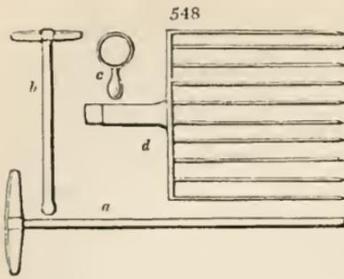
use of a pronged shovel, fourteen inches square, which may be universally recommended for this purpose (*fig. 548. d*). His large hammer (*a*), small one (*b*), and gauge for the size of the broken stone (*c*), are in very general use, as well as the pronged shovel. Hammers may be made of cast iron, where the stones to be broken are about their own weight; the best shape is a narrow oval: the advantage of using cast iron is its cheapness. (*Farm. Mag. xxii. 159.*)
