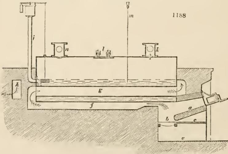
four times its diameter in length. Witty's patent gas-furnace is applied to *l*; *a* is the inclined plane; *b*, the fire-bars; *c*, the dead plate; *e*, the ash-pit. The flame and heated air passes under the boiler, through the bottom flue, *f*, thence through the tubular flue, *g*, right through the body of water in the
