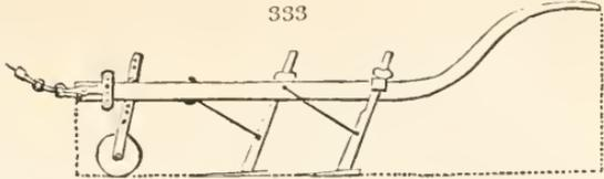
2672. *The Northumberland horse hoe* (see Report, &c. p. 43.) is of a triangular form, and contains three coulter and three hoes, or six hoes, according to the state of the soil.
