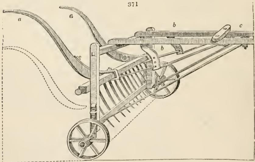
put in and out of gear by means of the handles (*a a*) and bent iron stays (*b b*). It is drawn by one horse in shafts (*c*), and is a very effective implement.
