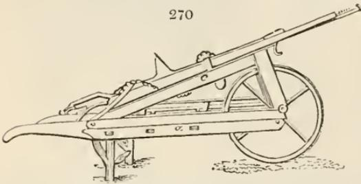
farmers in the neighbourhood of large towns. The apparatus, with every implement necessary to be used in cutting, weighing, and binding, may be packed together so as to form a wheelbarrow. (*fig. 270.*) When unpacked (*fig. 272.*), the wheel is taken out, and the bottom of the barrow (*a*) turned upside down upon the ground as a platform. (*fig. 271.*) The standard (*b*),
