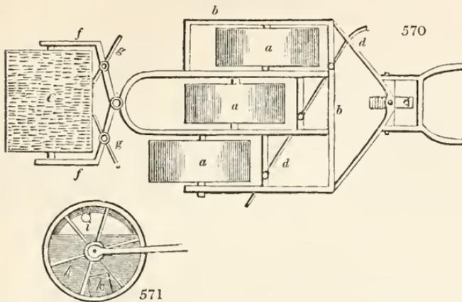
are the three cylinders for pressing the loose stones of the road together. As the apparatus is drawn along, these cylinders revolve upon their axes, which are mounted in the frame *b b b*. There is a small guide roller, or wheel in front of the frame to which the shafts are attached, and by which the apparatus may be turned round, or guided in a curved course; *d d* is a thin plate of iron placed obliquely across the machine, in front of the rollers; it is attached to the framing by rods and
