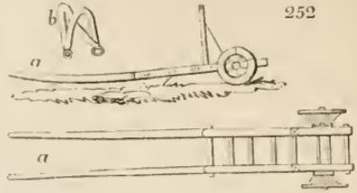
2543. *The truck* (fig. 253.) is a machine of the barrow kind for conveying compact heavy weights, such as stones, metals, &c.
