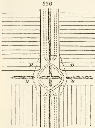
side of a hedge may be used as a road (fig. 536.), to avoid driving over a field in tillage. This may be easily effected by a few gates being placed in the line of the headland or nearly so, and not too near each hedge or to each other, so that a waggon may easily drive through them on the right or left, as the crops may require; a few hurdles (a) may guard each field in grain alternately, and will furnish a useful fold or enclosure to detain sheep, colts, &c.
