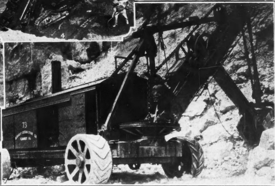
1. Loading in magnesite quarry with electrically operated shovel. 2. Gasoline-operated tractor shovel. 3. Stripping by steam shovel in gypsum quarry. 4. Loading sand in excavation work with portable bucket loader. 5. Loading gypsite with scraper. 6. Excavating a gold dredge pit with tractor and scraper. 7. Steam shovel with traction wheels
