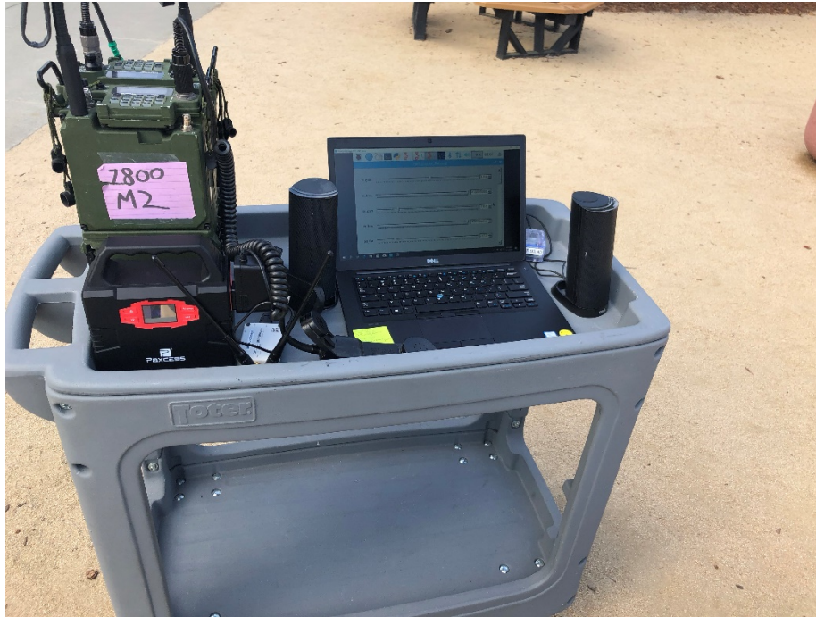
Figure 48. Radio Flow-Graph Verification Test Setup
