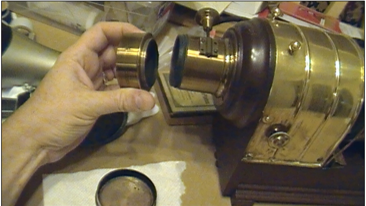
Lantern: All lens components were separated and cleaned.
