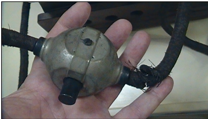
Lantern: On/Off switch.
