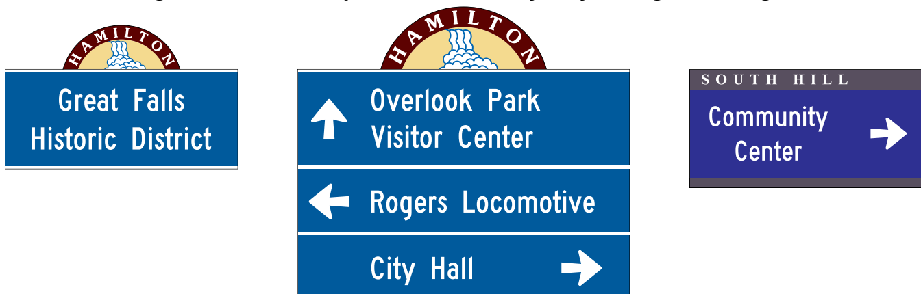
Figure 2D-30. Examples of Community Wayfinding Guide Signs
